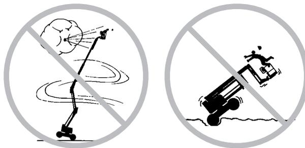
Use extreme care and slow speeds while driving the machine in stowed position across uneven terrain, debris, unstable or slippery surfaces and near holes and drop-offs.
