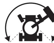
Note: When the drive enable system is in use, the machine may drive in the opposite direction that the drive and steer control handle is moved.
