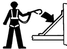
Occupants must wear a safety belt or harness and comply with applicable governmental regulations. Attach the lanyard to the anchor provided in the platform.
