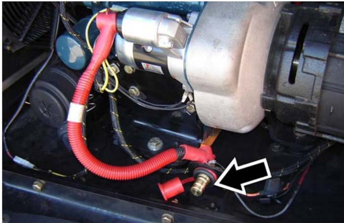
2. Connect the negative battery contact of the external battery to a grounded location on the machine.
