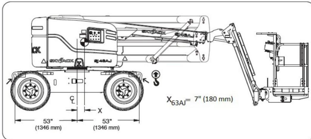
Figure 3-3d. Lifting Points (Model SJ63AJ)
