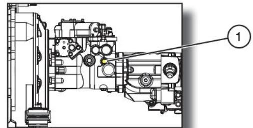
Figure 2-7b. Drive Bypass Valve (Model SJ63AJ)
