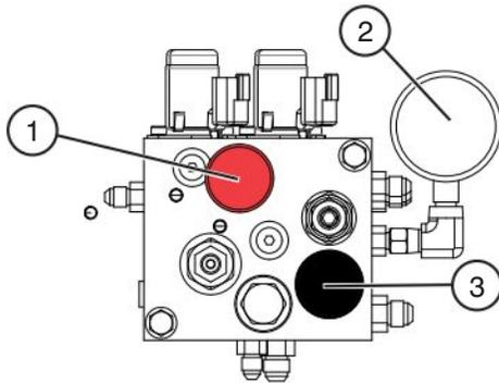
Figure 2-8b. Brake Manifold
