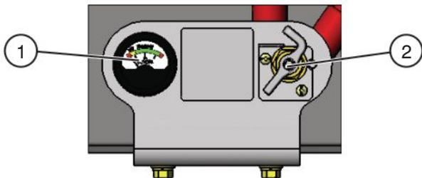
Figure 2-1. Main Power Disconnect Switch & Battery Charge Indicator
