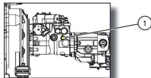
Figure 2-2b. Drive Bypass Valve (Model SJ63AJ)
