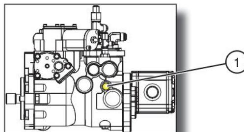
Figure 2-2a. Drive Bypass Valve (Models SJ46AJ & SJ51AJ)
