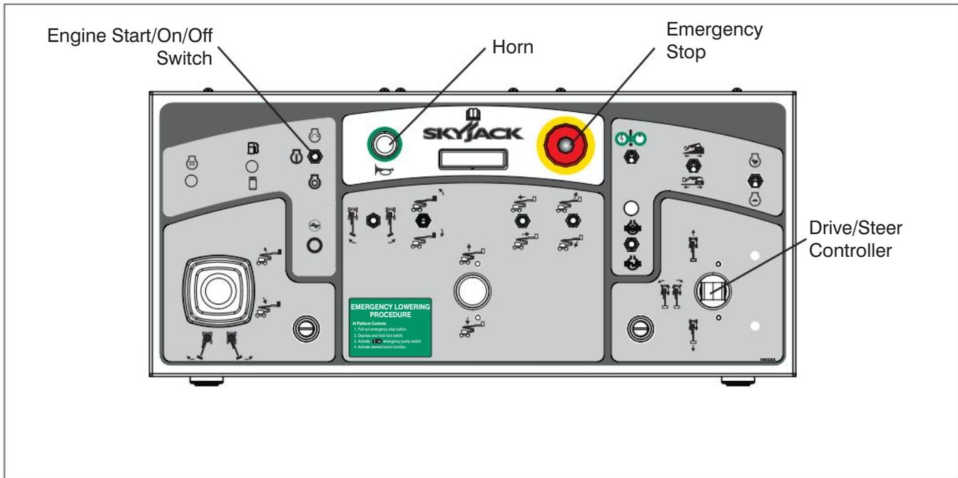
6. On platform control console, select “
