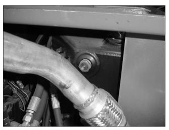
Figure 7 - Hydraulic Fluid Reservoir
