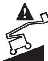
If the tilt alarm sounds when the platform is raised, the Machine Not Level indicator light will come on and the drive function in one or both directions will not operate. Identify the condition of the boom on the slope as shown below. Follow the steps to lower the boom before moving to a firm, level surface. Do not rotate the boom while lowering.
