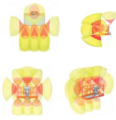
**Figure 29. SkySense Coverage Level 2 Areas (3-Bar)**
