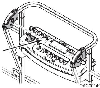
Operator passes through path of sensor beam.
