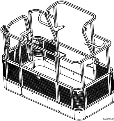
**Figure 22. Platform Mesh to Mid Rail**
