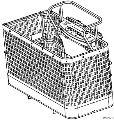
Figure 20. Fabric Mesh to Top Rail
