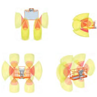
**Figure 28. SkySense Coverage Level 1 Areas (2-Bar)**
