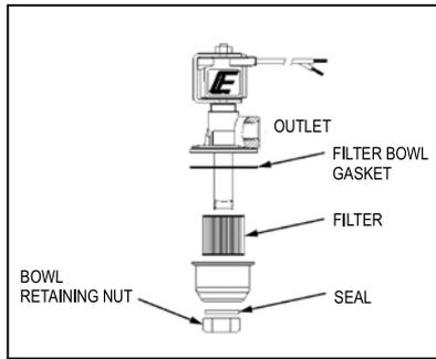
**Figure 33. Kubota Filter Lock Assembly**
