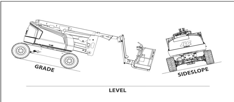
Figure 8. Grade and Side Slope
