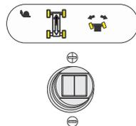
This machine is equipped with a Drive Orientation Indicator. The yellow light on the platform control console indicates that the boom is swung beyond the rear drive tires and the machine may Drive/Steer in the opposite direction from the movement of the controls. If the indicator is illuminated, operate the Drive function in the following manner:
