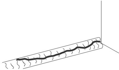
**Figure 3. Weld Crack**
