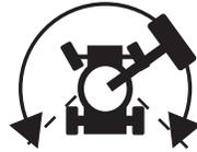
To drive, hold the drive enable switch to either side and slowly move the drive control handle off center.
