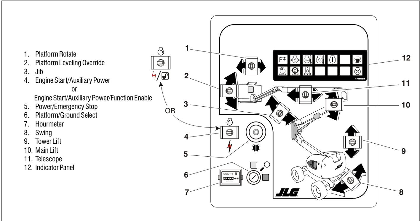
**Figure 3-1. Ground Control Station - AJ Models**
