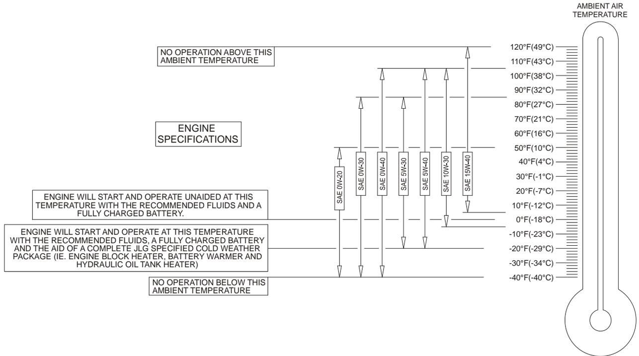
Figure 6-6. Engine Operating Temperature Specifications - Caterpillar - Sheet 1 of 2
