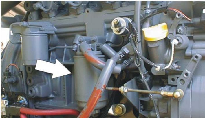
Lube Point(s) - Replaceable Element
