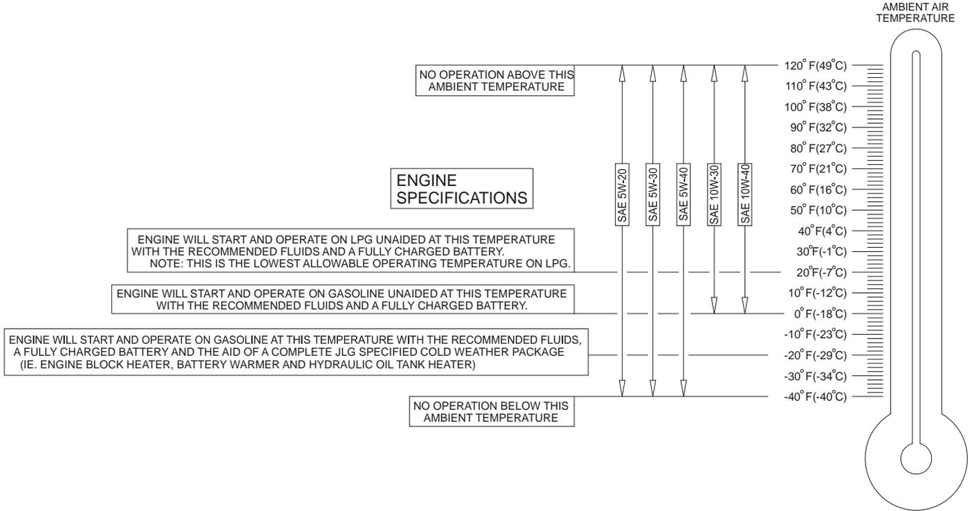
Figure 6-4. Engine Operating Temperature Specifications - Ford - Sheet 1 of 2
