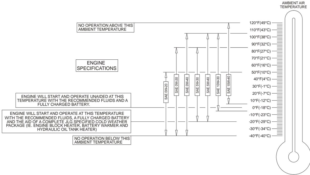
Figure 6-10. Engine Operating Temperature Specifications - Perkins - Sheet 1 of 2
