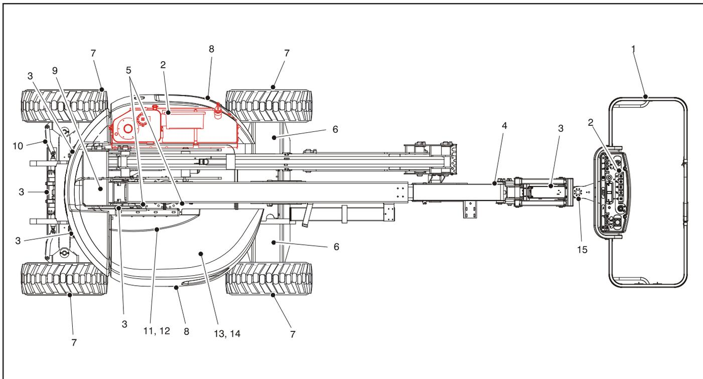
Figure 2-3. Daily Walk-Around Inspection - Sheet 1 of 3
