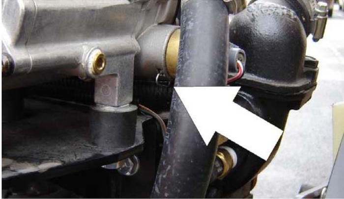
**NOTE:** Have a small container ready to collect oil that will drain freely from the regulator at this point.
