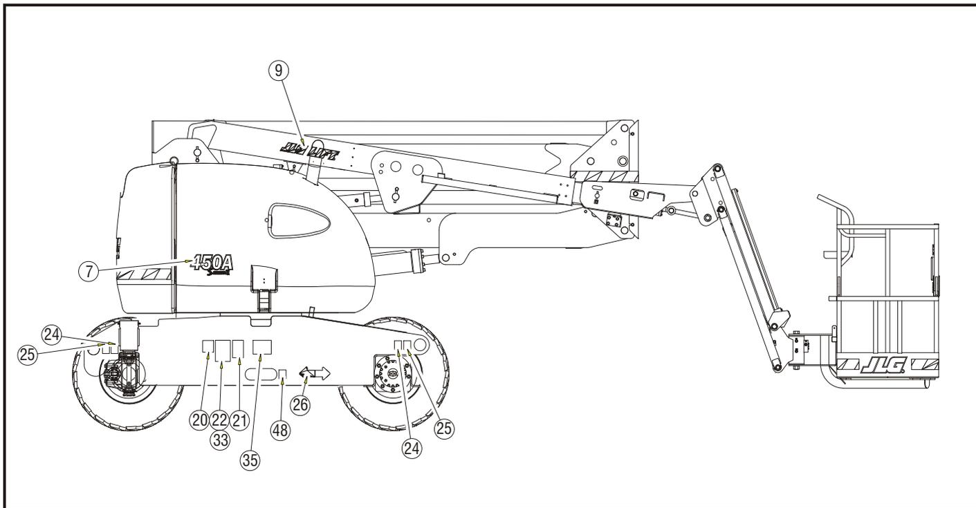
Figure 4-8. Decal Installation - Sheet 3 of 6
