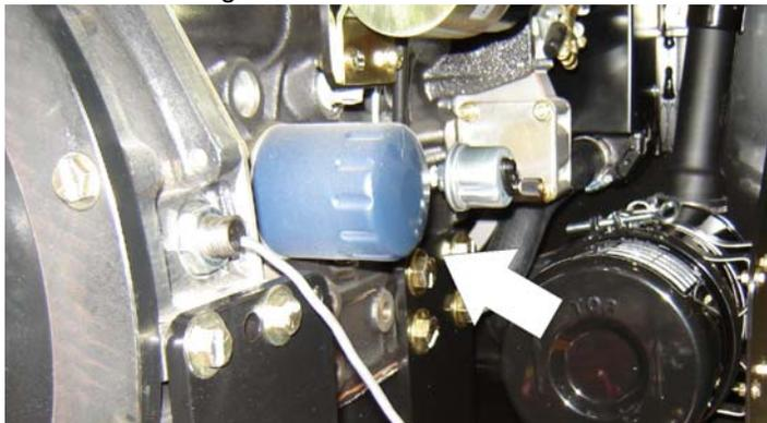
Lube Point(s) - Fill Cap/Spin-on Element (JLG P/N 7026855)
