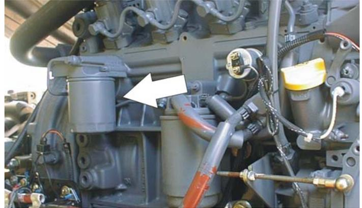
Fill Cap/Spin-on Element (JLG P/N 7016641)
