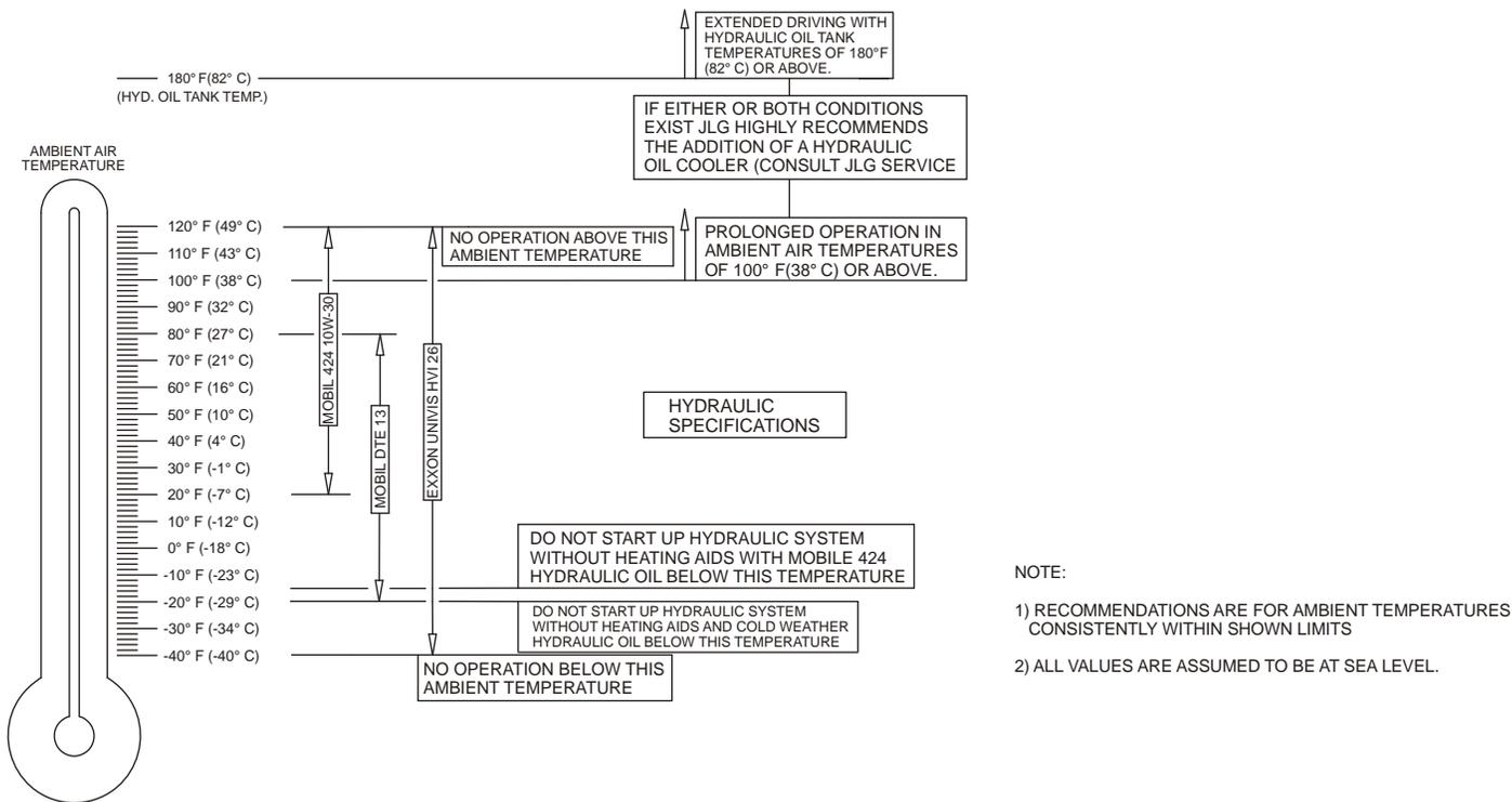
**Figure 6-9. Engine Operating Temperature Specifications - GM - Sheet 2 of 2**
