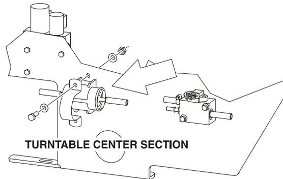
Lube Point(s) - Replaceable Element
