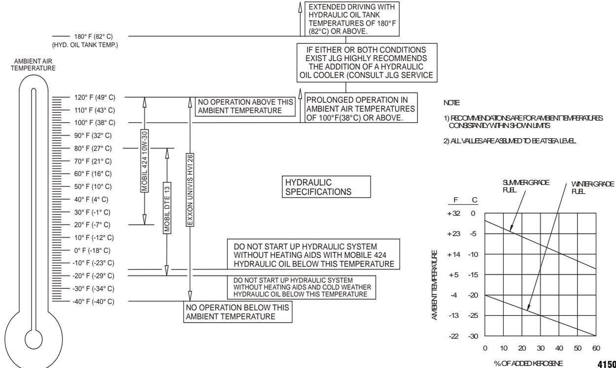
Figure 6-3. Engine Operating Temperature Specifications - Deutz - Sheet 2 of 2
