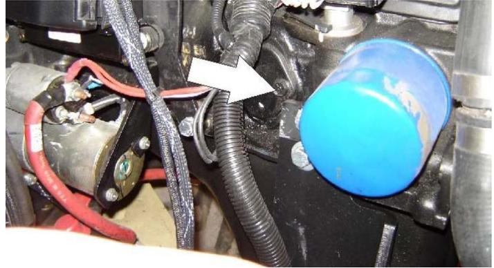
Lube Point(s) - Fill Cap/Spin-on Element (JLG P/N 7027965)
