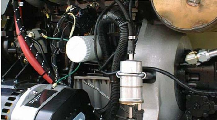
Lube Point(s) - Fill Cap/Spin-on Element (JLG P/N 7014501)
