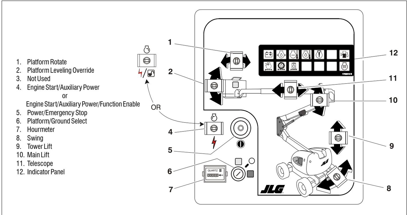
Figure 3-1. Ground Control Station - A Models
