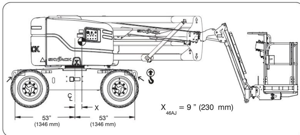
**Figure 10** Approximate center of gravity - SJ63 AJ
