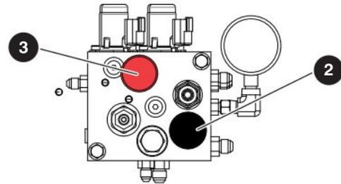
Figure 08 SJ63 AJ brake release system
