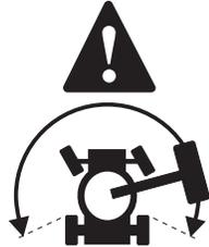
To drive, hold the drive enable switch to either side and slowly move the drive control handle off center.
