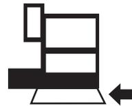
If the platform bumper comes into contact with an object, the machine will shut down and no functions will operate.
