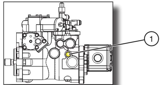
Figure 2-7a. Drive Bypass Valve (Models SJ46AJ & SJ51AJ)
