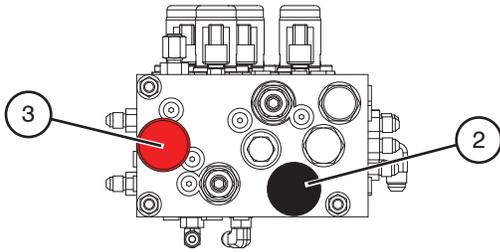
Figure 2-8a. Brake Manifold
