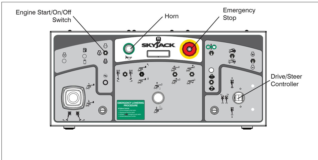
6. On platform control console, select “
