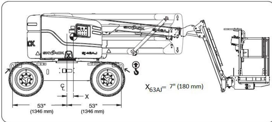
Figure 3-3d. Lifting Points (Model SJ63AJ)
