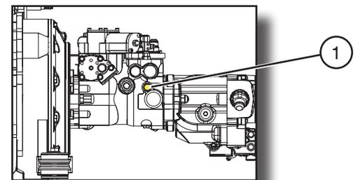
Figure 2-2b. Drive Bypass Valve (Model SJ63AJ)
