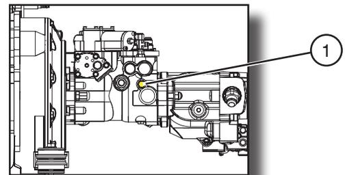
Figure 2-7b. Drive Bypass Valve (Model SJ63AJ)
