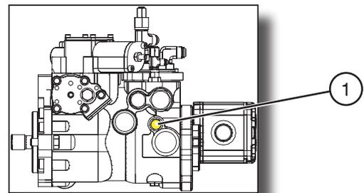
Figure 2-2a. Drive Bypass Valve (Models SJ46AJ & SJ51AJ)
