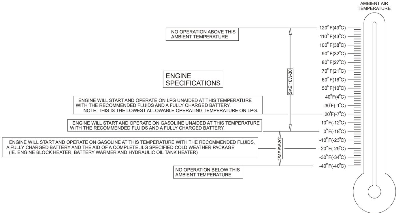
**Figure 7-3. Engine Operating Temperature Specifications - GM - Sheet 1 of 2**
