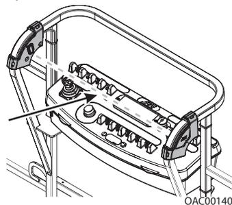
Operator passes through path of sensor beam.
