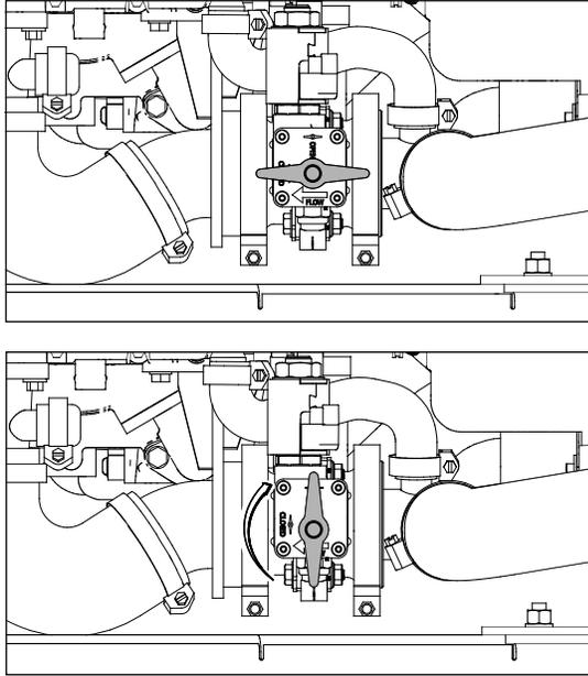
**Figure 4-4. ASOV Reset (Closed to Open Position)****Fuel Reserve / Shut-Off System**
