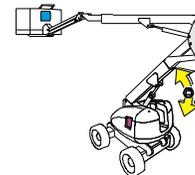
6. Lower the tower boom fully and continue to hold down the switch to Tower Down for an additional 20 seconds.
