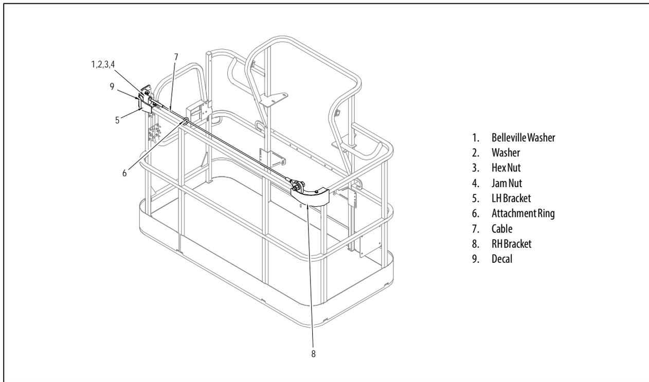
**Figure 6-2. Bolt-On External Fall Arrest System**
