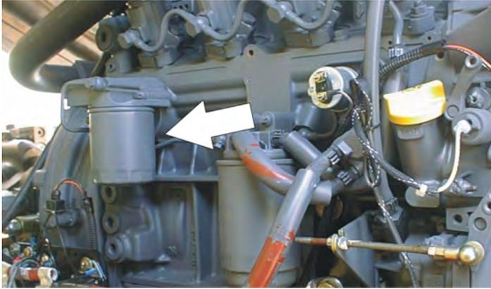
Lube Point(s) - Fill Cap/Spin-on Element
