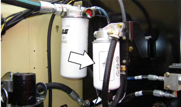
Lube Point(s) - Replaceable Element
