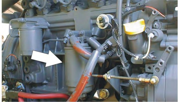
Lube Point(s) - Replaceable Element
