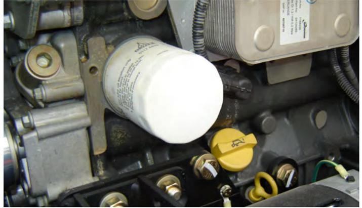
Lube Point(s) - Fill Cap/Spin-on Element
