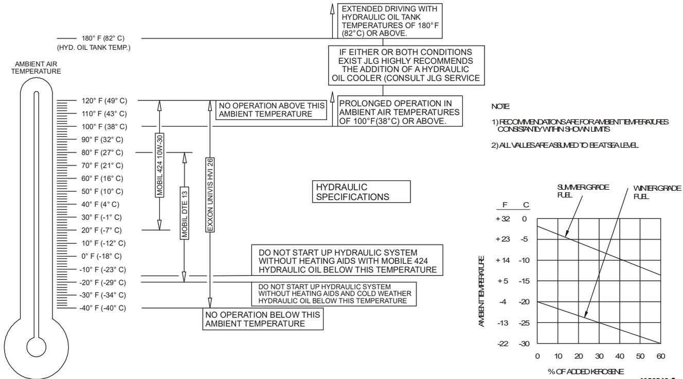
Figure 7-2. Engine Operating Temperature Specifications - Deutz - Sheet 2 of 2
