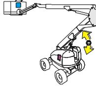
7. Repeat steps 3 thru 6 as necessary until the upright is 90° (vertical) relative to the chassis.
