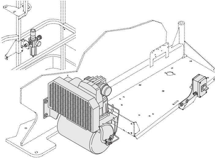
SkyAir™ supplies compressed air to the platform. A filter/regulator located in the platform controls air pressure. The on/off switch is located in the engine compartment. This accessory receives power from the SkyPower™ system.
