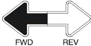
2. Push and release the Drive Orientation Override switch. Within 3 seconds, slowly move the Drive control toward the arrow matching the intended direction of machine travel. The indicator light will flash during the 3 second interval until the drive function is selected.
