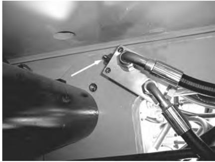
**Figure 3. Tower Boom Vertical Limit Switch**
