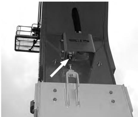
Figure 4. Tower Boom Horizontal Limit Switch
