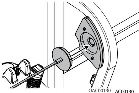
Reattach magnetic end of cable to bracket if it becomes disconnected.
