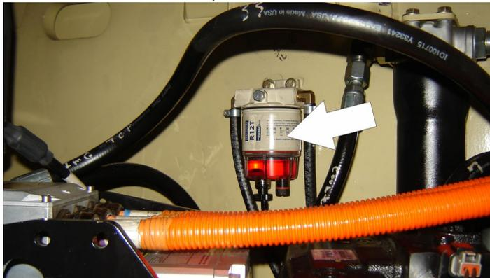
Lube Point(s) - Replaceable Element
