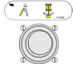
**NOTE:** Main boom lift and swing functions may be selected in combination. Maximum speed is reduced when multiple functions are selected.
