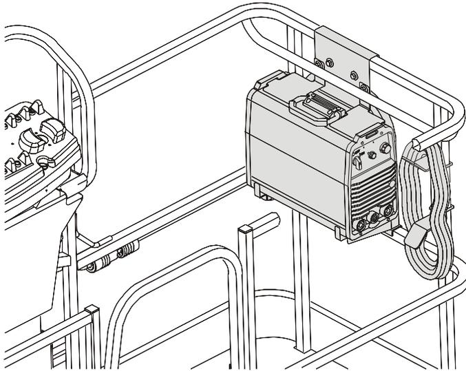
SkyWelder™ is capable of TIG and Stick welding, producing 200 Amps at 100% duty cycle or 250 Amps at 50% duty cycle. This accessory receives power from the SkyPower™ system.
