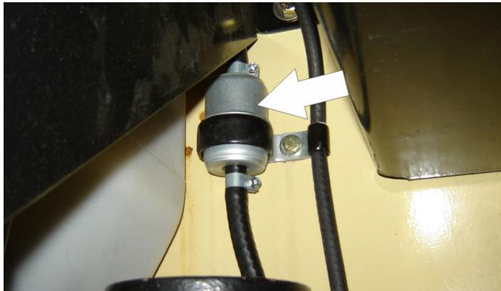
Lube Point(s) - Replaceable Element
