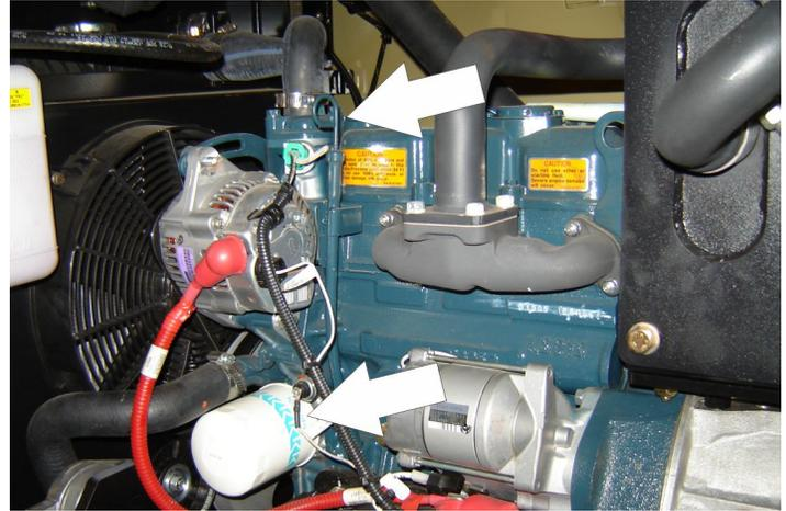
Lube Point(s) - Fill Cap/Spin-on Element
