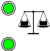
tery packs are, the faster it will blink. When the battery packs are close to being balanced and is equalizing, the light will blink green.
