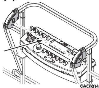
Operator passes through path of sensor beam.
