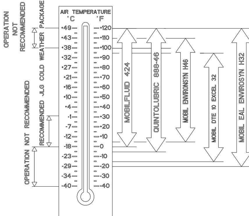
**Figure 7-2. Hydraulic Oil Operating Temperature Specifications - Sheet 1 of 2**
