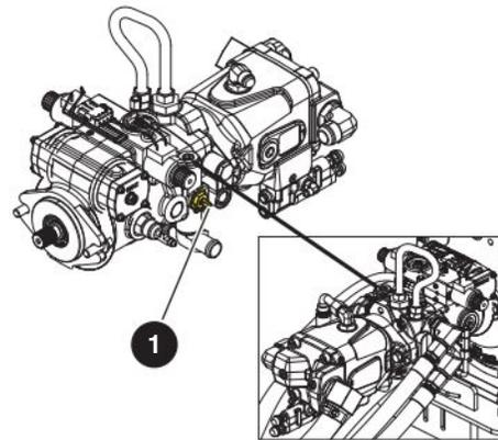
Figure 21 Drive Bypass Valve
