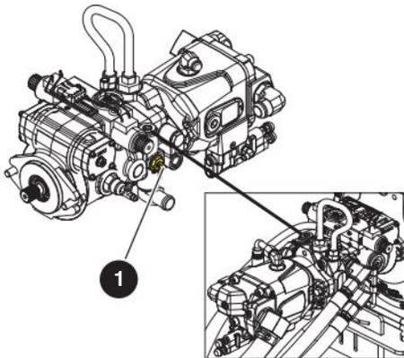
Figure 22 Drive Bypass Valve
