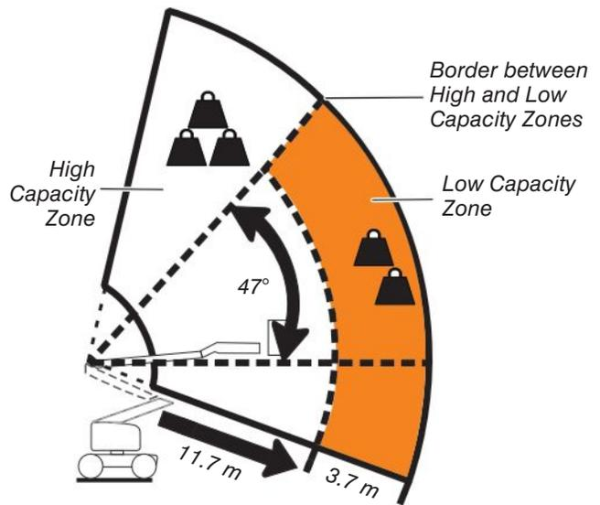
Figure 11 High and Low Capacity Zones
