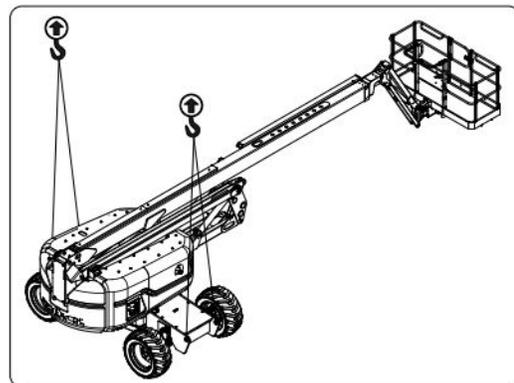
Figure 28 Lifting Points
