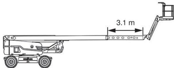
Figure 12 Fly Boom Extension into Low Capacity Zone
