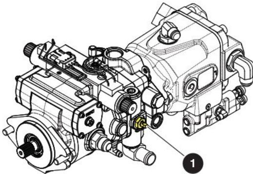
Figure 15 Drive Bypass Valve
