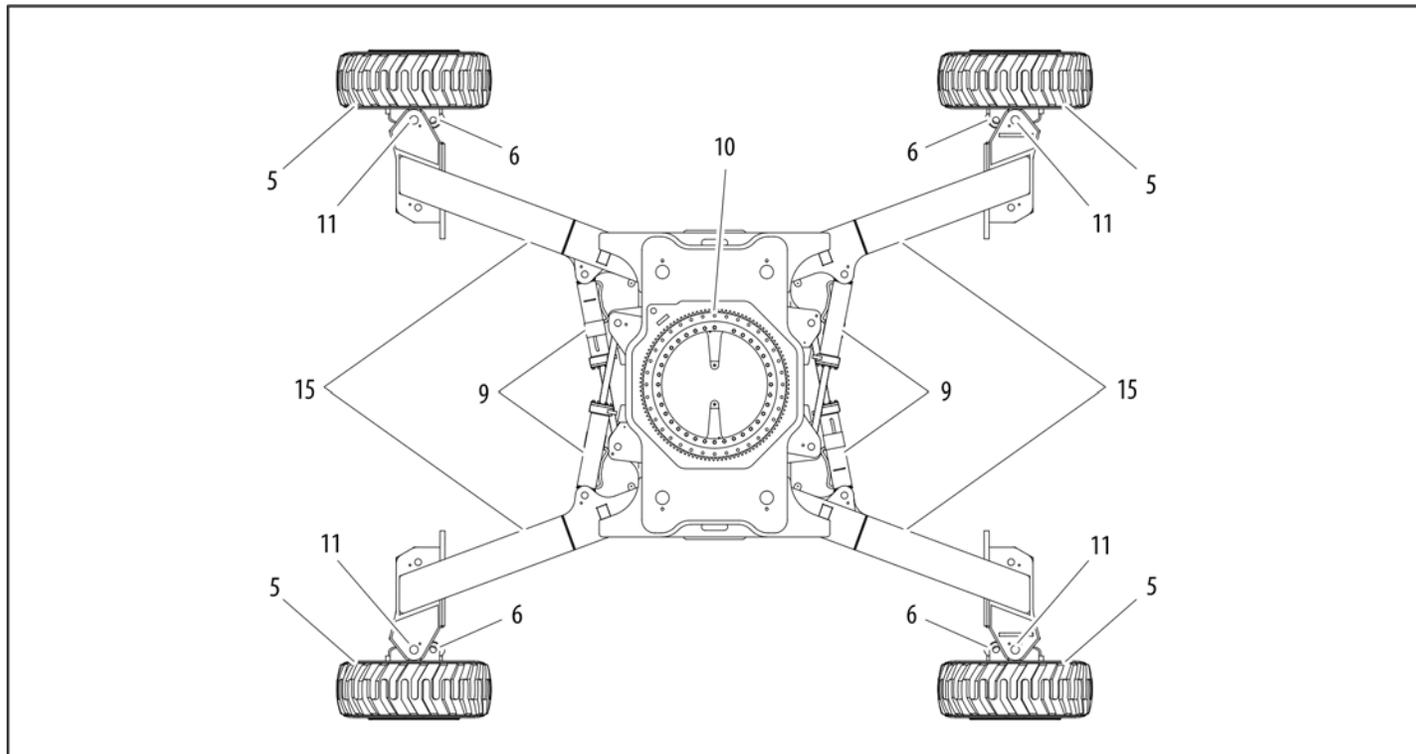
**Figure 2-6. Daily Walk-Around Inspection - Sheet 3 of 5**
