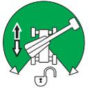
When the boom is swung over the rear tires or further in either direction, the Drive Orientation indicator will illuminate when the drive function is selected. Push and release the switch, and within 3 seconds move the Drive/Steer control to activate drive or steer. Before driving, locate the black/white orientation arrows on both the chassis and the platform controls. Move the drive controls in a direction matching the directional arrows for the intended direction of travel.
