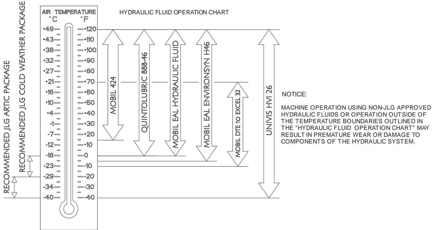
**Figure 7-2. Hydraulic Oil Operation Chart - Sheet 1 of 2**
