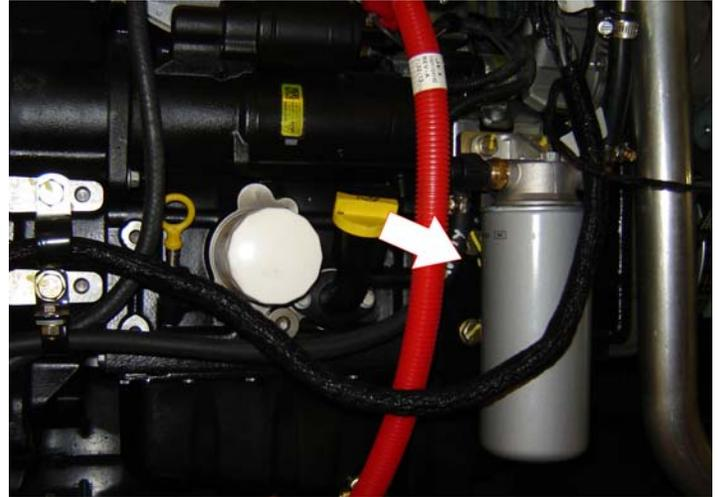
Lube Point(s) - Replaceable Element
