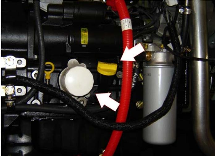
Lube Point(s) - Fill Cap/Spin-on Element
