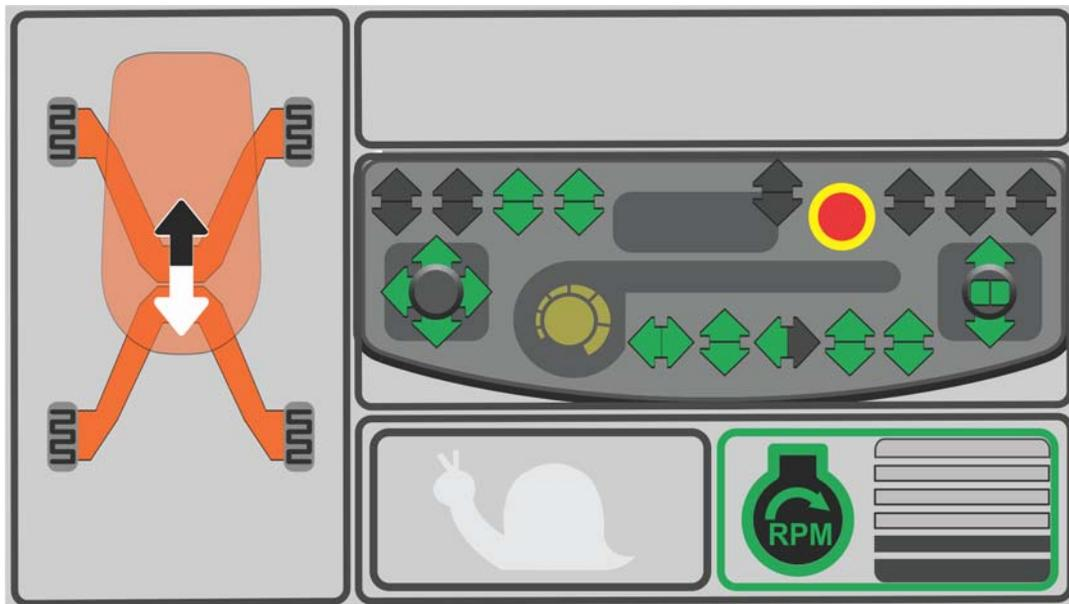
**Figure 5-21. Axles Extended Screen**
