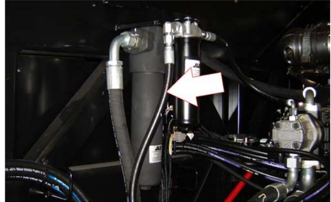
Lube Point(s) - Replaceable Element
