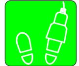
Releasing the footswitch removes power from all controls and applies the drive brakes.
