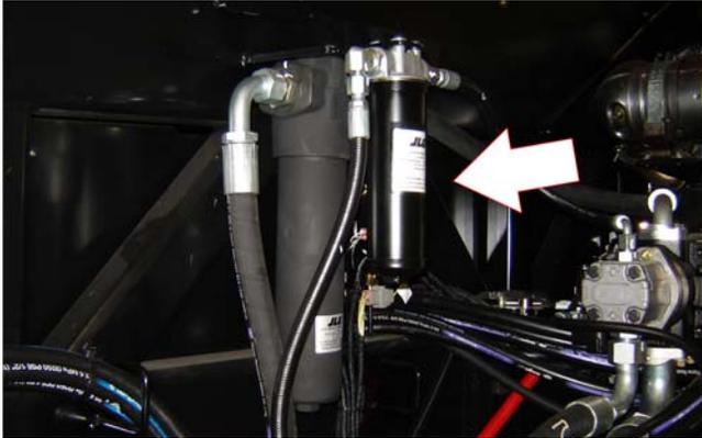
Lube Point(s) - Replaceable Element
