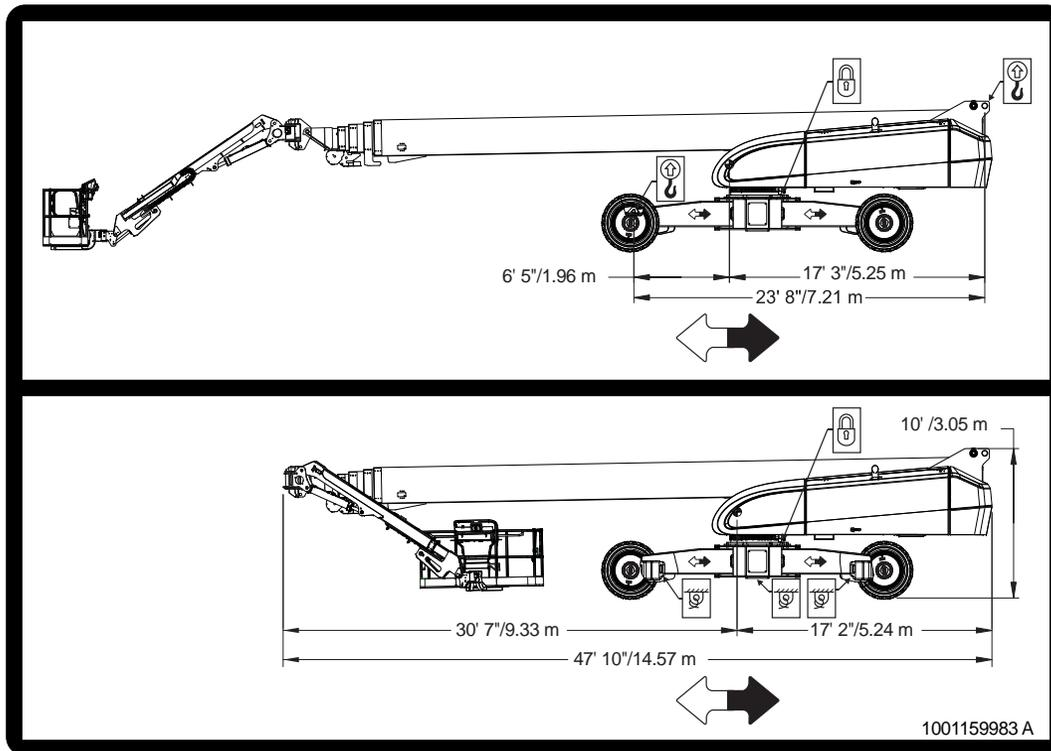
**Figure 4-7. Lifting and Tie Down Chart**
