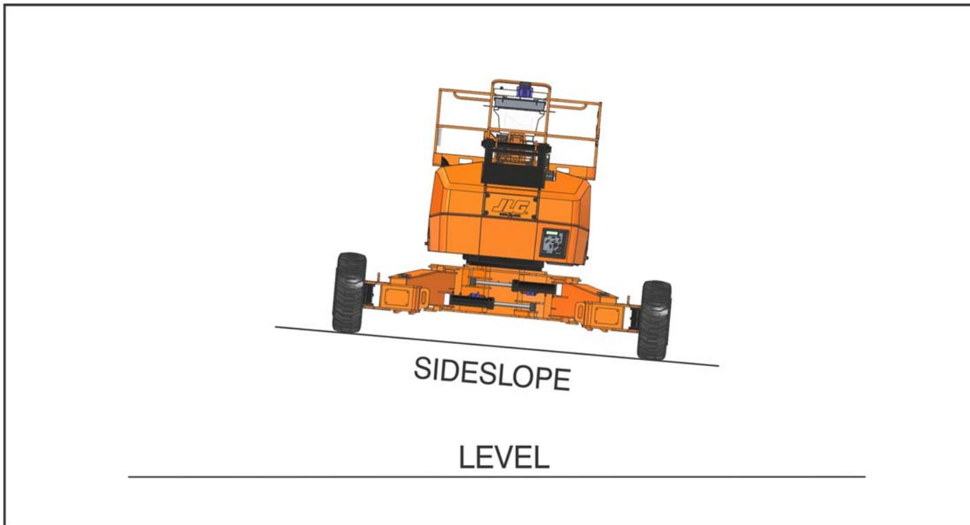
**Figure 4-4. Grade and Side Slopes - Sheet 2 of 2**
