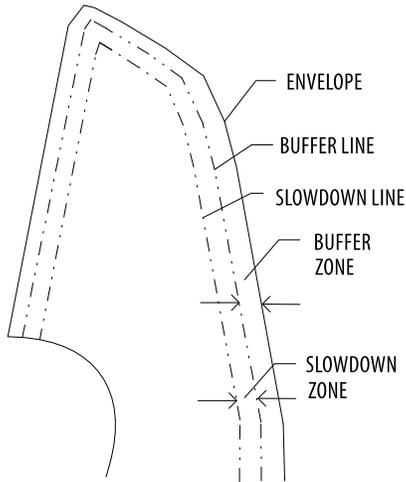
When the platform approaches the edges of the operating envelope all machine functions are slowed down except jib and platform functions, telescope in or out at the rearward edge and telescope in or out on the forward edge are slowed down automatically by the boom control system to reduce machine motions.
