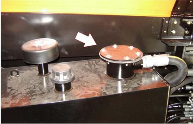
Lube Point(s) - Replaceable Element
