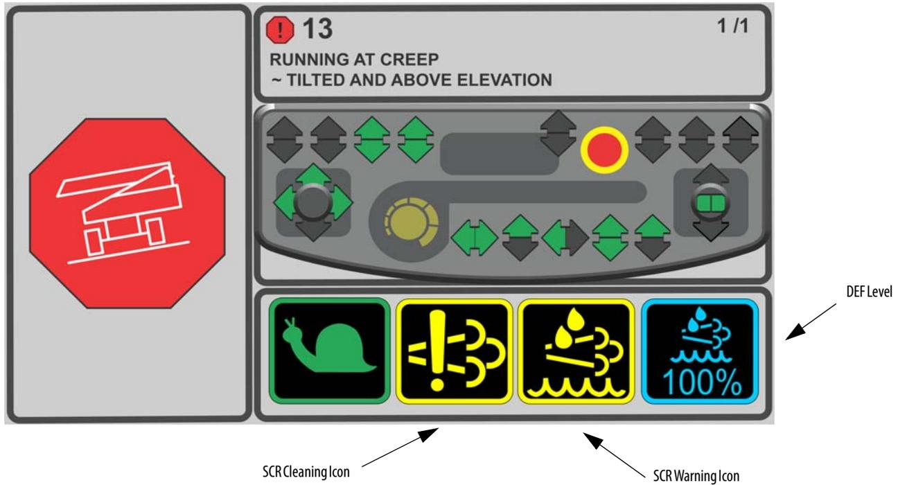
Figure 5-27. SCR Cleaning Screen - Sheet 1 of 2
