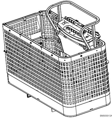
Figure 29. Fabric Mesh to Top Rail
