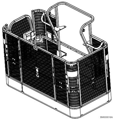
**Figure 33. Platform Mesh to Top Rail**
