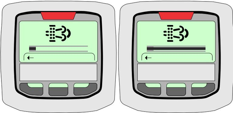
5. After the cleaning process is complete, the engine will run for approximately 5 minutes to allow the engine and Exhaust After Treatment (EAT) to cool down. The Indicator Gauge will display the "Regen Complete" screen as shown and the Emissions Temperature indicator will no longer be illuminated.
