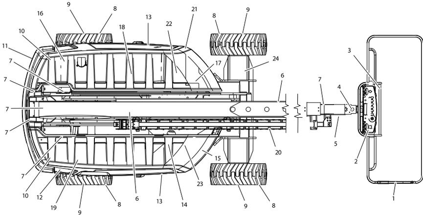
Figure 5. Daily Walk-Around Inspection Diagram
