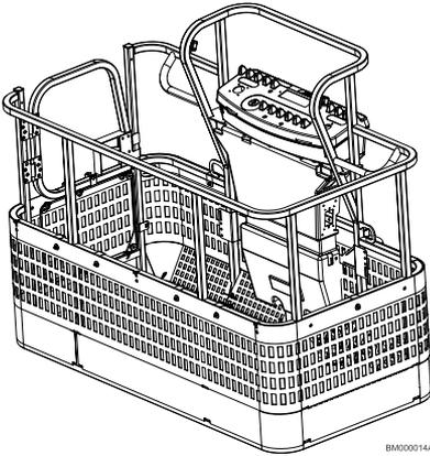
Figure 28. Fabric Mesh to Mid Rail
