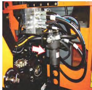
**Figure 49. Platform Filter — SJ Models**
