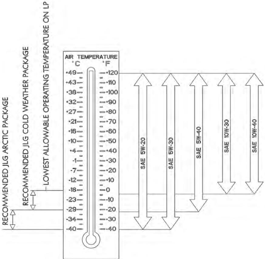
Figure 45. Engine Oil Operating Temperature Specifications - Ford MSG425
