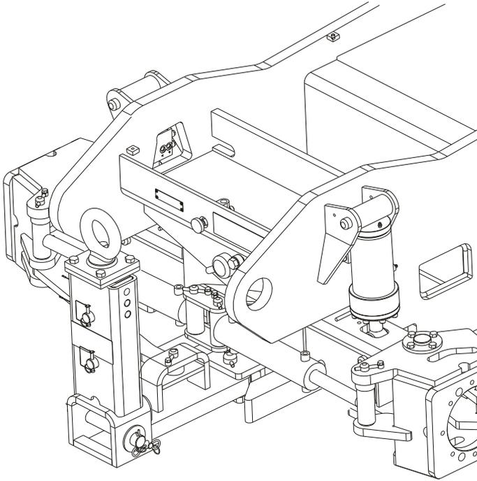
**Figure 18. Towbar (Raised Position)**
