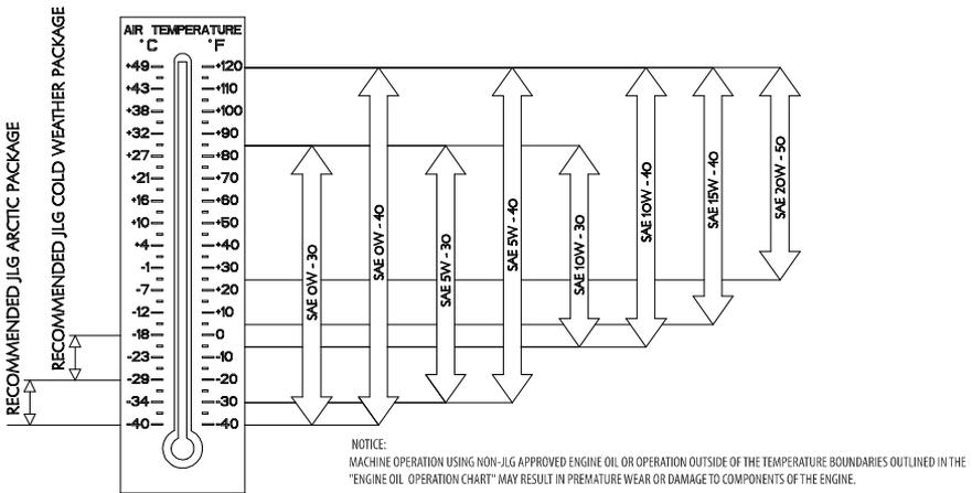
Figure 44. Engine Oil Operating Temperature Specifications - Deutz 2011
