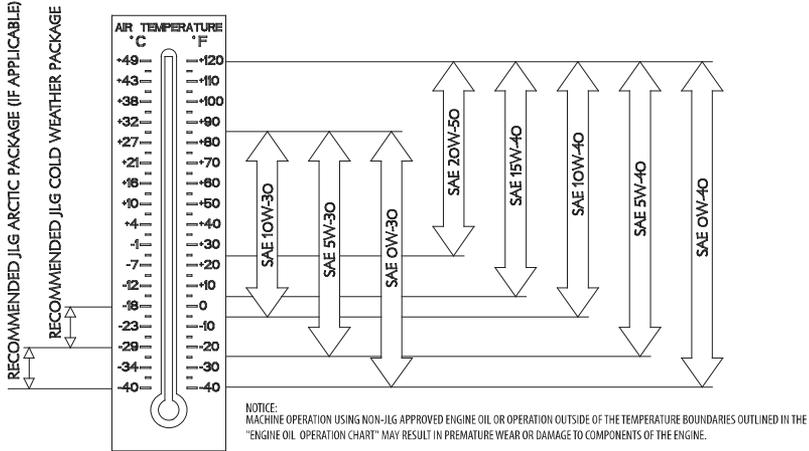
Figure 43. Engine Oil Operating Temperature Specifications - Deutz 2.9L
