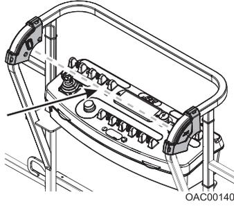
Operator passes through path of sensor beam.
