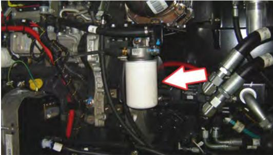
12. Fuel Pre-Filter - Deutz D2.9/TD2.9, 2.2L Stage V
