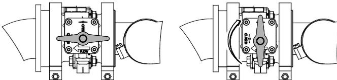
**Figure 12. ASOV Reset (Closed to Open Position)**
