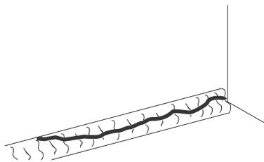
**Figure 4. Weld Crack**
