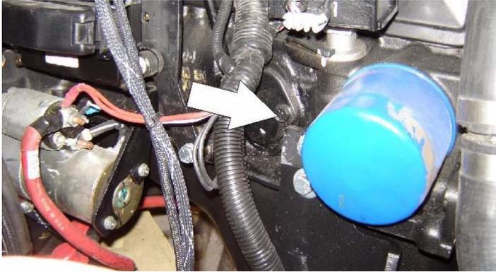
Lube Point(s) - Fill Cap/Spin-on Element
