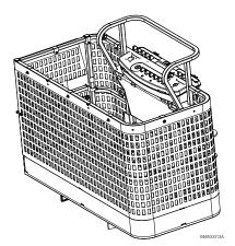
Figure 27. Fabric Mesh to Mid Rail
