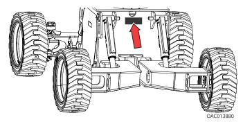
Figure 41. Serial Number Plate
