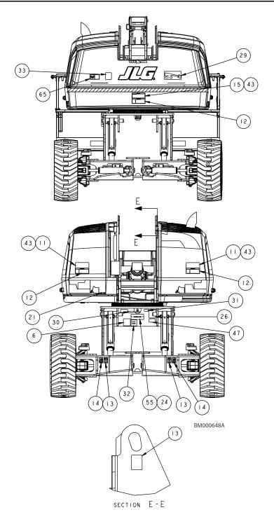
Figure 20. 670SJ Self Leveling Decals - 2 of 4 31221364
