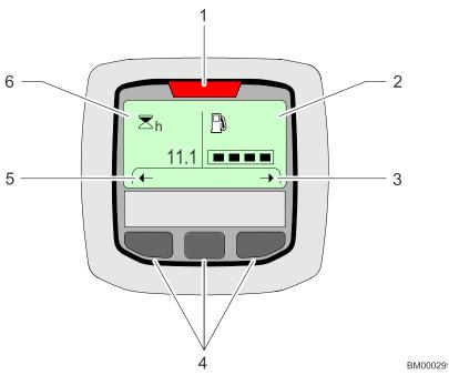
**Figure 8. Ground Control Console Display Gauge**
