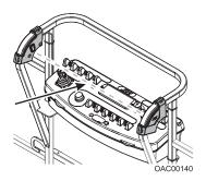
Operator passes through path of sensor beam.
