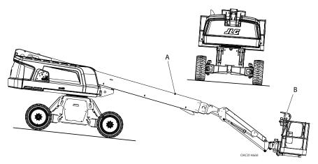
Figure 14. Traveling with Boom in Stowed Position — Auto Level Not Active
