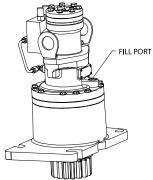
Wheel Drive Hub Lube Point(s) - Level/Fill Plug Capacity - 24 oz. (0.7 L) Lube - 80w90 Gear Oil
