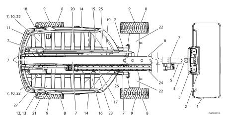
Figure 4. Daily Walk-Around Inspection Diagram
