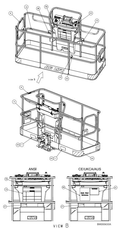
Figure 22. 670SJ Self Leveling Decals - 4 of 4 31221364
