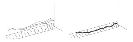
Figure 2. Parent Metal Crack
