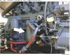
Oil Change with Filter - Deutz 2.9, 2.2L Stage V Lube Point(s) - Fill Cap/Spin-on Element Capacity - 9.5 Quarts (9.0 L) Crankcase Lube - EO
