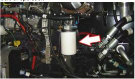
Fuel Pre-Filter - Deutz D2.9/TD2.9, 2.2L Stage V Lube Point(s) - Replaceable Element Interval - Drain water daily; Every year or 600 hours of operation
