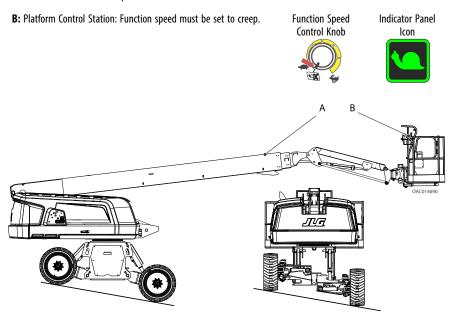
Figure 13. Traveling with Boom out of Stowed Position — Auto Level Active
