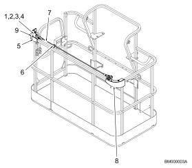
Figure 24. Bolt-On External Fall Arrest System
