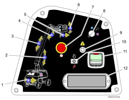
670SJ Self Leveling Ground Control Station — With MSSO
