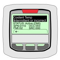
Figure 7. Engine Diagnostic Screen
