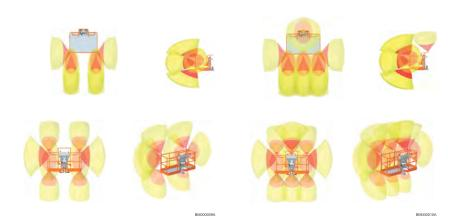
Figure 37. SkySense Coverage Level 1 Areas (2– Bar)
