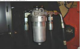
Hydraulic Return Filter Interval - Change after first 50 hours and every 6 months or 300 hours thereafter or whenever Charge Filter is replaced
