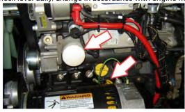
Fuel Filter - Deutz 2.9, 2.2L Stage V Lube Point(s) - Replaceable Element Interval - 600 hours of operation
