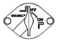
Figure 15. Battery Disconnect Switch
