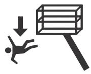
During operation, occupants in the platform must wear a full body harness with a lanyard attached to an authorized lanyard anchorage point. Attach only one (1) lanyard per lanyard anchorage point.
