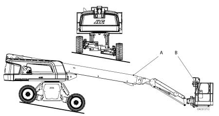
Figure 12. Traveling with Boom in Stowed Position — Auto Level Active
