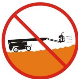
Reduce the transfer speed according to the conditions of the ground, the traffic, the slopes, presence of workers or other factors which can cause collisions.
