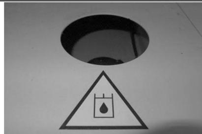
Note: The hydraulic oil should be applied to the local environment, and be filtered at the accuracy of 20  $\mu$  m.
