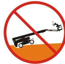
Make sure the ground is able to support the weight of the machine indicated in the technical specifications in the Manual. Do not use the machine on muddy, icy, slippery, uneven ground or where there are holes in the ground.
