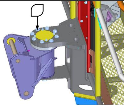
Check if there is some bolts is slacken or missing and the sensor undamaged. If there is abnormal condition, ask for help from DingLi or your agency.
