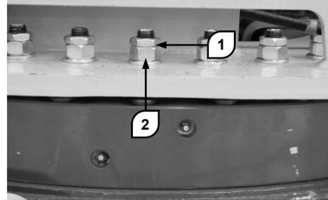
Check the turret fixing nuts on the slewing ring gear. Check for rusted, slackened or missing nuts.
