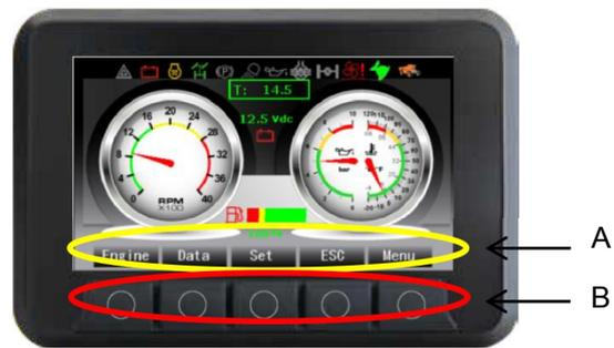
This panel contains the basic information for monitoring the working of the truck. The pages and options available are displayed in the lower part of the screen [A] and are controlled by the corresponding buttons present below [B].
