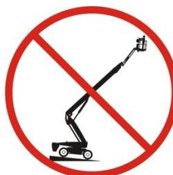
Do not raise or extend the boom unless the machine is placed on a stable level surface.
