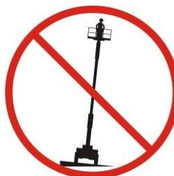
Never exceed the maximum permitted inclination of the truck; the maximum permitted inclination of the truck is indicated in the technical specifications and on the ID plate on-board the machine.
