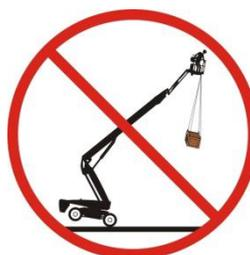
Do not position or fix weights or loads projecting from any part of the machine.
