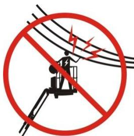
Observe the local and national regulatory standards in force concerning the distance required from electricity lines. At least the safety distance indicated in the Table below must be respected.
