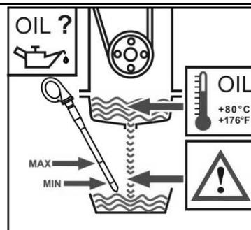
An insufficient and/or excessive lubricant oil level can damage the engine. Check the oil level only with the engine horizontal and stopped. Check the lubricant oil level only while it is warm, 5 minutes after the engine is switched off. Do not remove the oil level rod with the engine running. Danger of burns.
