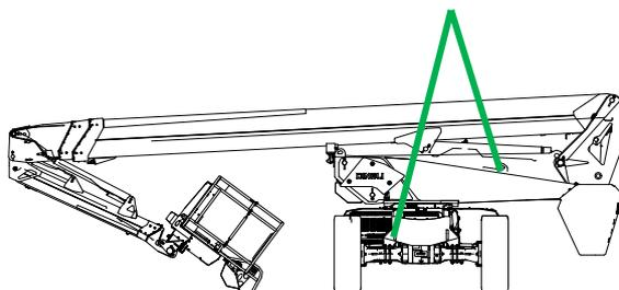
Adjust the lifting devices in such a way as to keep the machine level and without causing damage to it.
