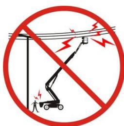
Move away from the machine in case of contact with live electricity lines. Workers on the ground or on the platform must not touch or operate the machine until the electric power supply has been disconnected.
