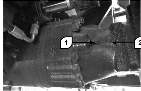
Go under the vehicle near the rear axle. Unscrew lock nut 1 of power screw 2. Tighten the power screw to fit flush to disengage the negative command brake. Repeat the operation for other three screws on the same axle. And then repeat the operation for front axle.
