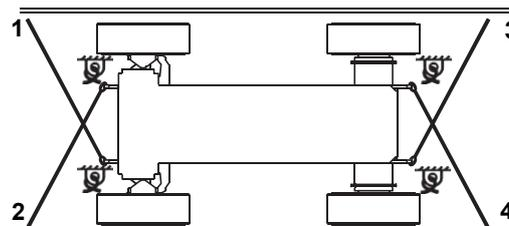
Use all four fixing devices provided on the chassis according to the diagram shown above.
