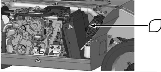
To remove dust and debris from the radiator mass, compressed air, pressurised water or steam can be used. However, it is preferable to use compressed air.
