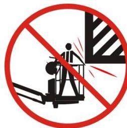
Take extreme care while gripping the platform railing to prevent danger of crushing.
