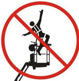
Do not sit, stand or climb on the railings of the platform. Always maintain a stable position on the platform foot board.
