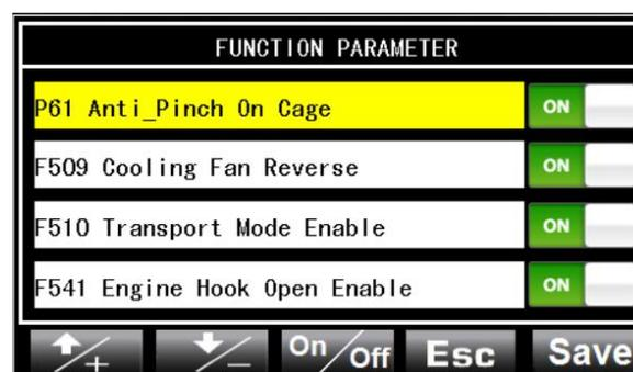
A Depressing or is used to choose the item separately. For example “P61 Anti\_Pinch On Cage”, “F509 Cooling Fan Reverse”, “F510 Transport Mode Enable” and “F541 Engine Hook Open Enable”. The chosen item would be shown in yellow background.
