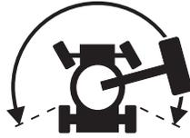
To drive, hold the drive enable switch to either side and slowly move the drive control handle off center.
