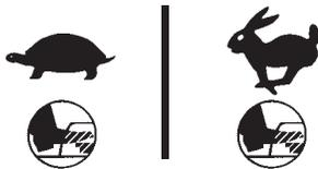
When the foot switch is not pressed, the engine will idle at the lowest rpm.
