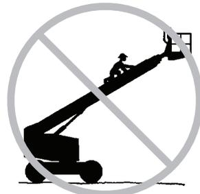
Do not enter or exit the platform unless the machine is in the stowed position and the platform is at ground level.
