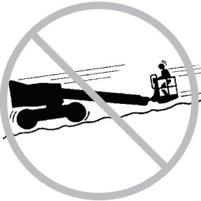
Do not operate a boom in the path of any crane unless the controls of the crane have been locked out and/or precautions have been taken to prevent any potential collision.
