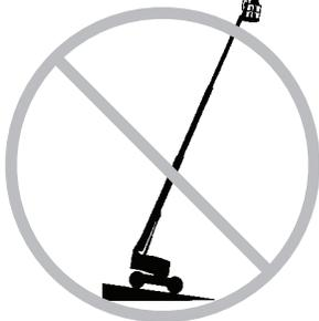
If the tilt alarm sounds when the platform is raised: Use extreme caution. Identify the condition of the boom on the slope. Follow the steps to lower the boom before moving to a firm, level surface. Do not rotate the boom while lowering.
