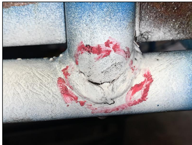
Photos 5 to 8 – Overview cracking found on basket frame
