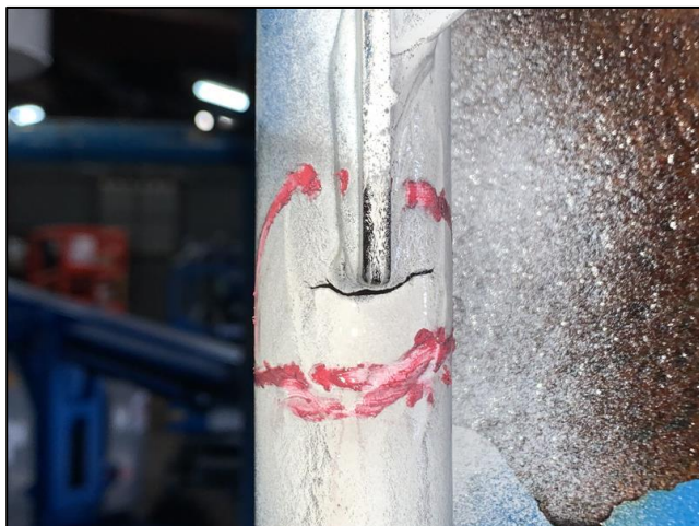
Photos 5 to 8 – Overview cracking found on basket frame
