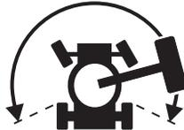
⦿ Result: The drive enable indicator light should come on and remain on while the boom is anywhere in the range shown.
