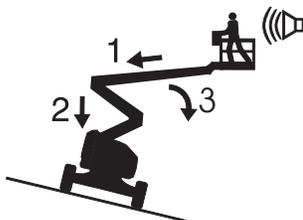
Do not raise the boom when wind speeds may exceed 28 mph / 12.5 m/s. If wind speeds exceed 28 mph / 12.5 m/s when the boom is raised, lower the boom and do not continue to operate the machine.
