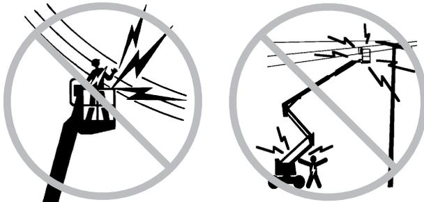
Maintain required clearances from electrical power lines and apparatus in accordance with applicable governmental regulations and the following chart.
