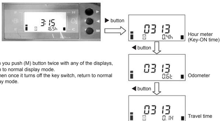
※ When you push (M) button twice with any of the displays, return to normal display mode.
