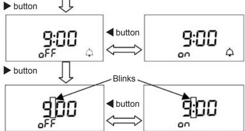
※ Push (M) button when the setting is completed, return to normal display mode.
