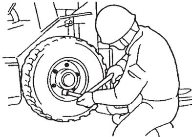
3. Check on the damage, cracks or abnormal wear of tires.
