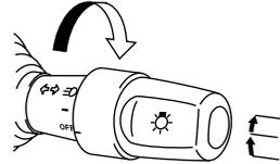
If the operator keeps the light “ON” and turn off the key, warning alarm sounds to prevent battery discharge.
