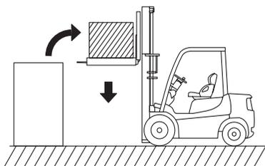
6. Lower the fork to about 15 to 20 cm from the ground and tilt the mast backward to make the load stable. Then, travel to the destination.
