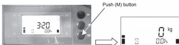
When the vehicle is stopped the load scale display appears. When the vehicle is traveling the speedometer display appears. The display changes automatically in the load scale display appears. This continues until the key switch is turned OFF.
