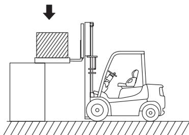
5. Fully insert the forks again, raise the load approx. 5 to 10cm and slowly back away. Then, lower the load to a safe height.
