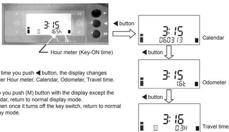
Each time you push ◀ button, the display changes in order Hour meter, Calendar, Odometer, Travel time.
