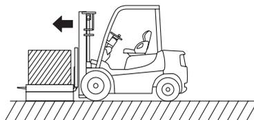
5. Hold the load by putting it against the backrest and then lift the fork 15 to 20cm from the ground. Then, tilt the mast back as much as possible.
