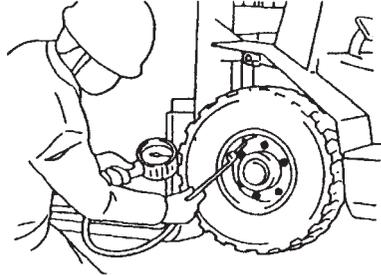
2. Check for loose hub nuts and tighten uniformly.
