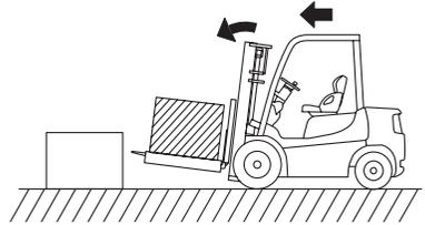
3. Tilt the fork to the vertical position, and lift to a position slightly higher than the place where the stack is to be placed.
