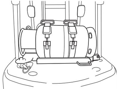
3. Check the bolts on the container fixing frame for looseness and the hose connections, etc., for looseness.
