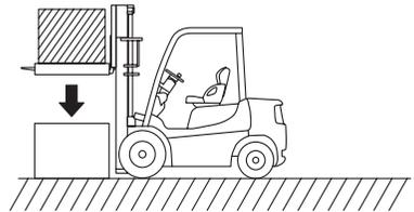
5. Gradually pull out the forks so as to not snag the load.
