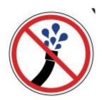
It is forbidden to flush the forklift with water pipe.
