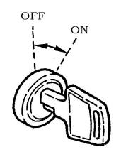
Removing the key prevents the truck from being switched on by unauthorised personnel.
