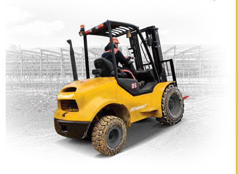
Two-Wheel Drive Rough Terrain Forklift 2,500 - 3,500 kg
