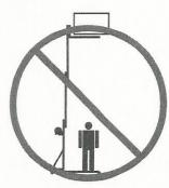
NEVER operate the material lift on a moving or mobile surface, such as a truck bed.
