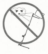
**NEVER** apply an additional side load or horizontal force to a material lift that is loaded or raised. **NEVER** place ladders or scaffold against the material lift.
