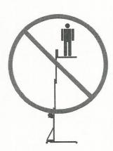
**NEVER** operate the material lift unless the legs and stabilizers are fully lowered and locked and all casters are in contact with the ground.
