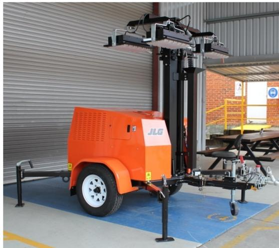
9. Raise the front of the machine by adjusting the front outrigger jacks until the machine is level and each outrigger support jack is pressing firmly against the ground, about two turns after contact with the ground. Do not attempt to raise the lighting tower by overextending the jack leg.
