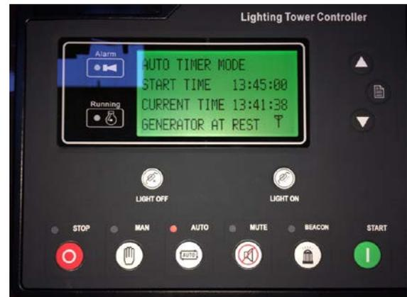
14. 10 seconds before the engine start-up an audible alarm sounds.
