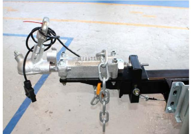
The tow ball coupling fitted to trailer axles with cable operated disc and drum brakes.
