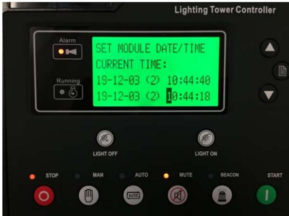
6. Set the time using the UP /DOWN arrows. Press MENU/CONFIRM to advance to the next place in the 24 hour clock (HR/MIN/SEC).
