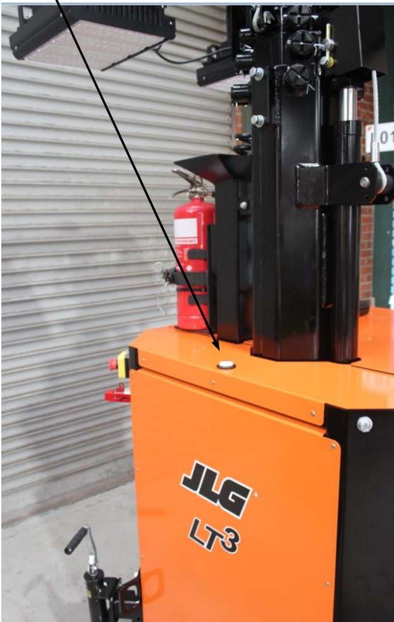
Fig 1.4.4 Bubble-Level Location
