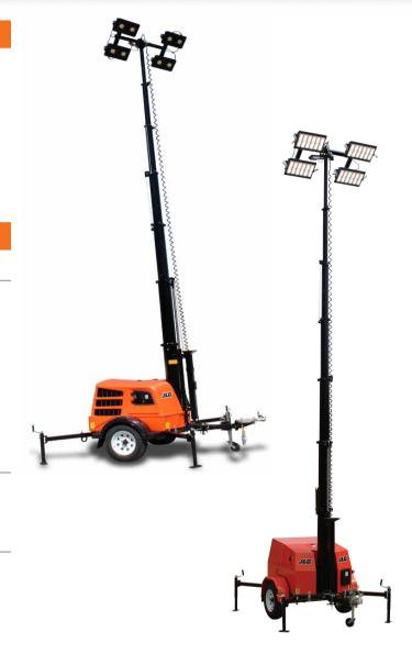
This 9 m tower features 4 x LED lights on a 48 V 'extra low voltage' system and weighs just 1100 kg, enabling easy one person set-up. Designed and manufactured in Australia the Metro-LED tower provides the value you need without sacrificing performance and quality you require.
