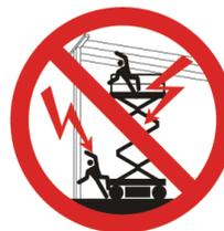
Keep a minimum safe distance from sources of high-voltage power.
