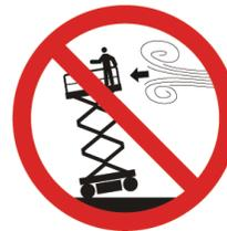
**DO NOT** raise the platform or operate elevated in windy or gusty conditions that exceed the limits specified in [section 7.4](#).
