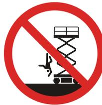
Prevent falling from the platform. Always keep a firm footing on the platform floor when working thereon. Do not climb on the toe-board, mid-rail, or top-rail. Do not use planks, ladders, or any other devices on the platform for achieving additional height or reach.
