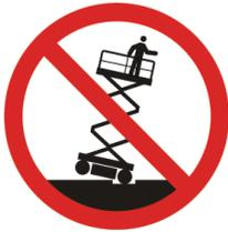
**DO NOT** drive elevated near depressions or holes of any type, loading docks, debris, drop-offs or surfaces that may affect the stability of the MEWP.
