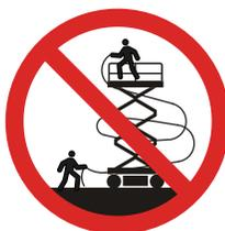
**DO NOT** allow the entanglement of ropes, cables or hoses with the MEWP, adjacent structures or objects.
