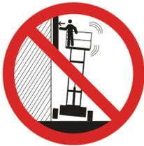
**DO NOT** exceed the maximum side force on the platform capacity label when elevated (refer to [section 7.4](#)).
