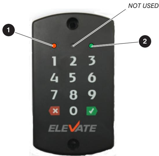
Figure 02 Keypad of the access control unit
