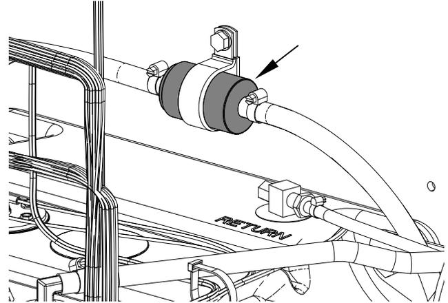
**NOTE:** Mounted inside fuel/hydraulic cabinet on left-rear cabinet wall behind fuel tank.
