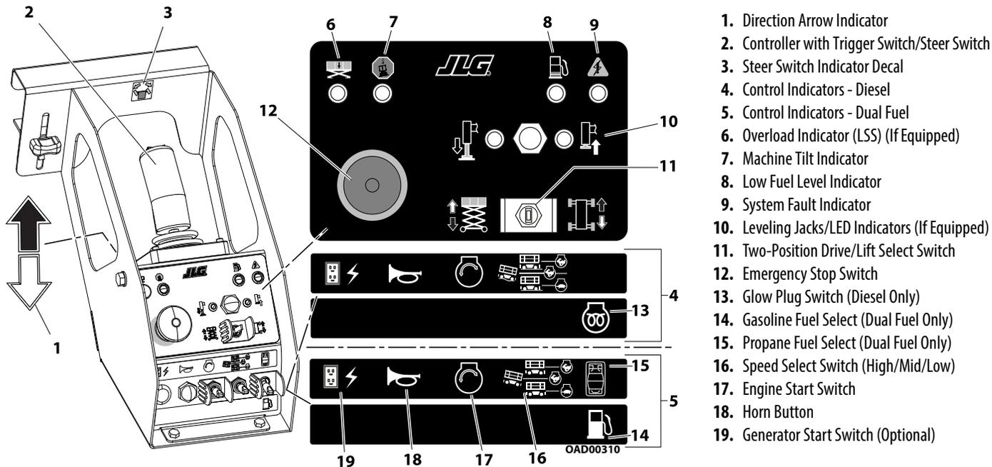
**Figure 3-4. Platform Control Station (Prior to SN 0200267916)**
