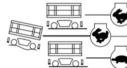
When platform is elevated above high drive cutout height, drive speed is reduced to (0.5 mph) regardless of Drive Speed Switch setting.
