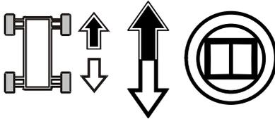
After selecting the drive function, depressing the trigger switch and moving the control handle forward will drive the machine forward and moving the control handle backwards will drive the machine backward.
