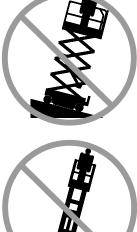
Do not raise the platform unless the machine is on a firm. level surface.
