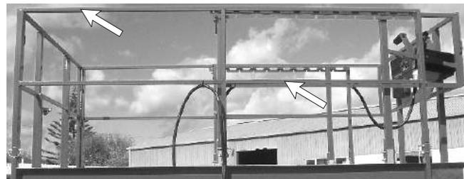
**Figure 2.5 - Fall Restraint**
