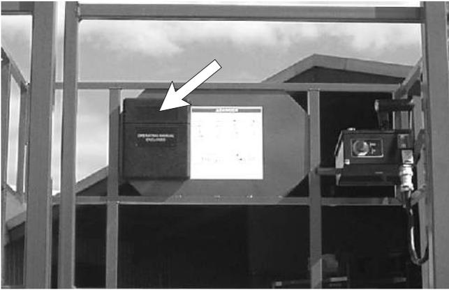
**Figure 7.34 - Operator Manual Holder**
