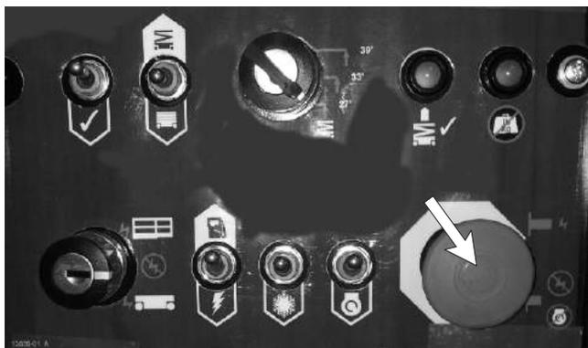
Figure 9.2 - Ground Control Box Emergency Stop Switch
