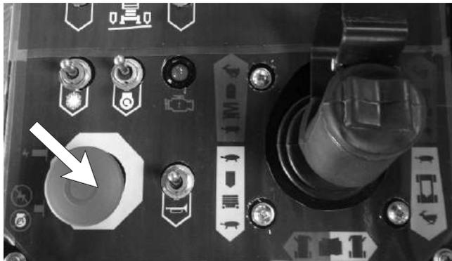
**Figure 2.1 - Platform Control Box Emergency Stop Switch**
