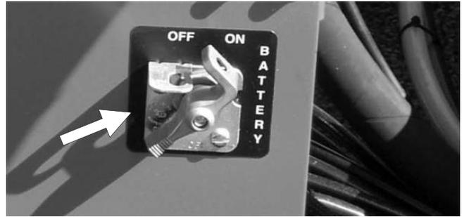
**Figure 6.2 - Battery Switch**
