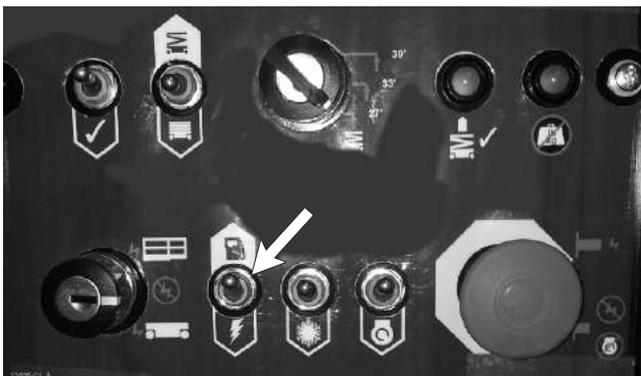
**Figure 11.2 - Diesel/Electric Selection Switch**
