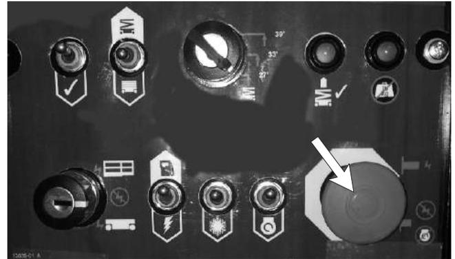
**Figure 2.2 - Ground Control Box Emergency Stop Switch**
