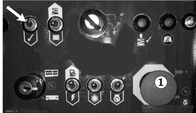
Figure 2.12 - Enable Switch
