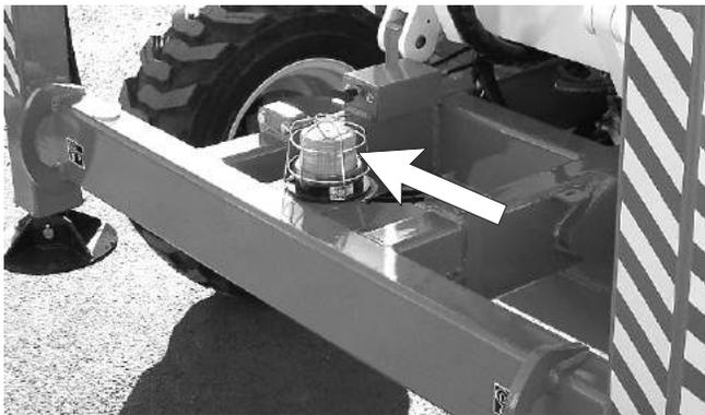
Figure 7.27 - Flashing Light
