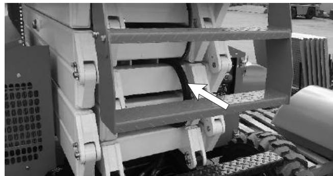
**Figure 7.11 - Wiring Harness in the Scissor Stack**
