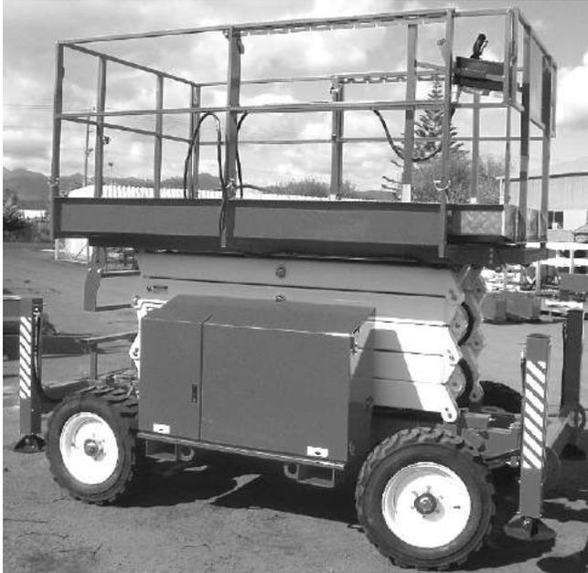
**Figure 10.1 - Correct Stowed Position**
