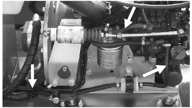
**Figure 7.5 - Fuel Leaks in Hoses & Joints**
