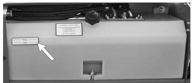
**Figure 4.4 - Hydraulic Oil Level**
