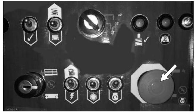
Figure 8.1 - Emergency Stop Switch at Ground Control Box
