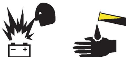
Batteries contain acid. Always wear protective clothing and eye wear when working with batteries.
