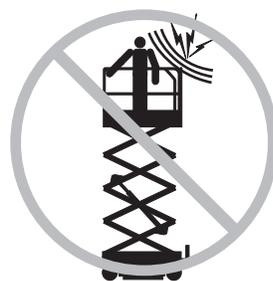
Keep away from the machine if it contacts energized power lines. Personnel on the ground or in the platform must not touch or operate the machine until energized power lines are shut off.
