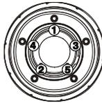
4. Tighten bolts in stages. Following the recommended sequence, tighten each bolt per wheel torque of 163 Nm (120 ft.lb.).
