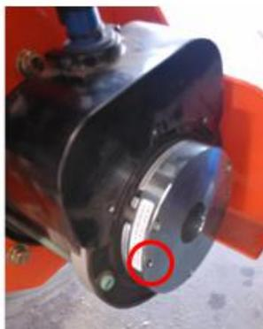
③ Turn the bolt clockwise. When the brake clearance is greater than 0.003in (0.08 mm), the brake is released.
