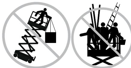
Do not put ladders or scaffolding within the platform or any part near the machine.
