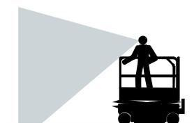
Pay attention to the range of sight and the existence of blind spots when the machine is started or operated.
