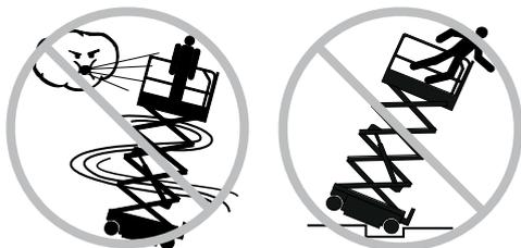
Do not operate the machine during strong winds or gusts. Do not increase the surface area of platform or load. Increasing the area exposed to wind will reduce the machine stability.
