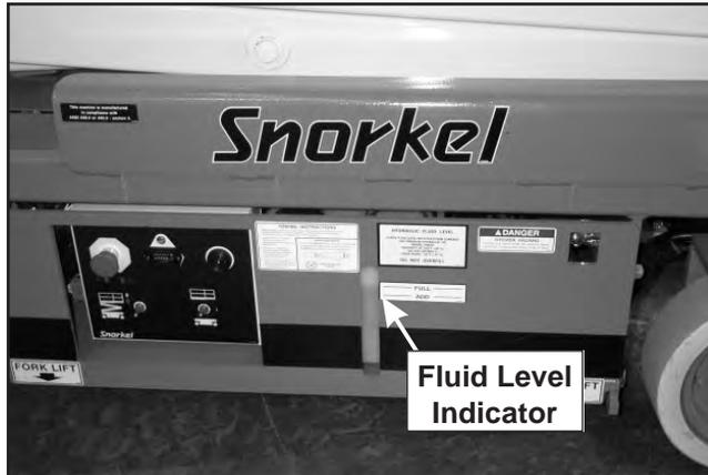
Figure 8.6—Fluid Level Indicator
