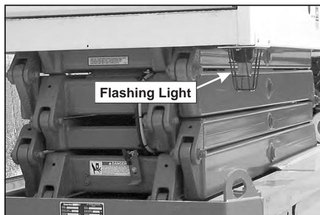
Figure 4.9—Flashing Light
