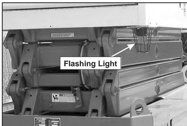
Figure 8.16—Flashing Light
