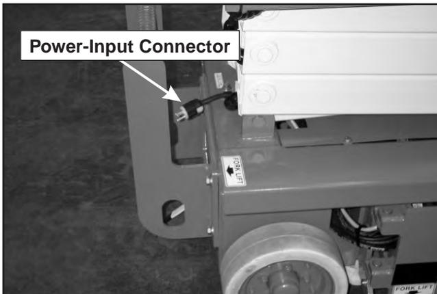
**Figure 9.7—Power-Input Connector**
