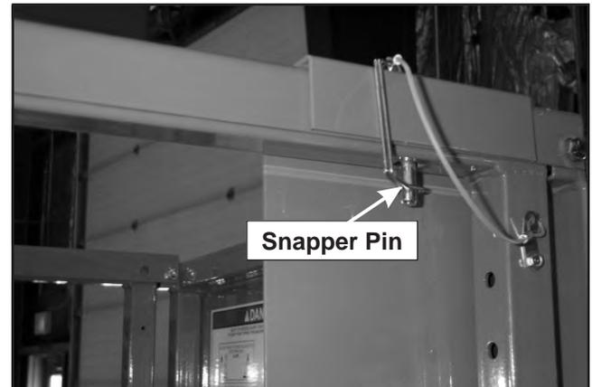
**Figure 8.20—Platform Extension Snapper Pin**
