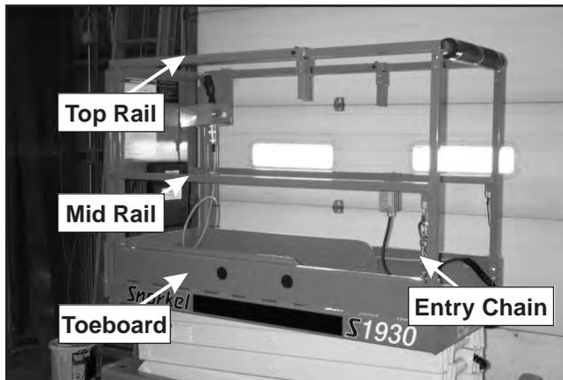
**Figure 8.19—Guardrail System**
