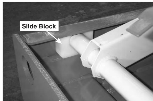
Figure 8.17—Scissors Arm Slide Blocks
