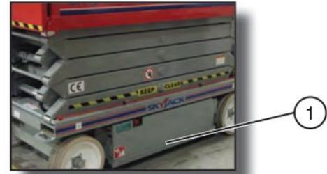
Figure 3-3. Pothole Protection Device
