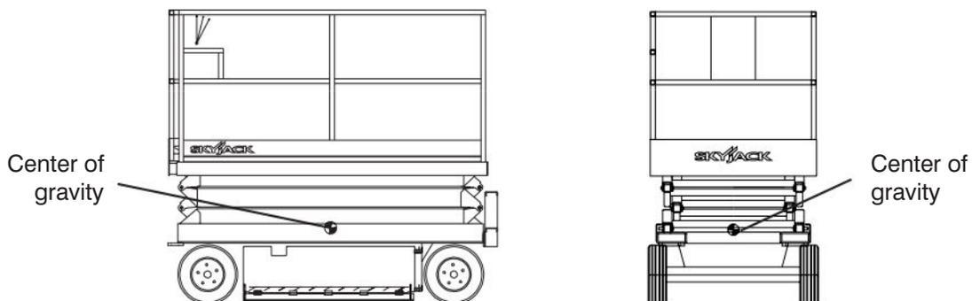
Figure 3-14. Center of Gravity
