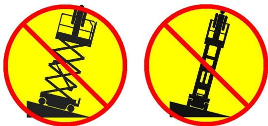
Do not depend on the tilt alarm as a level indicator. The tilt alarm sounds on the chassis and in the platform when the machine is on a slope.
