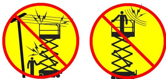
Maintain safe distances from electrical power lines and apparatus in accordance with
