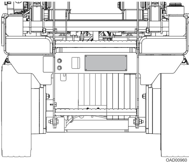
**Figure 10. 2632 Serial Number Plate**
