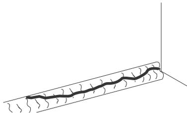
**Figure 2. Weld Crack**
