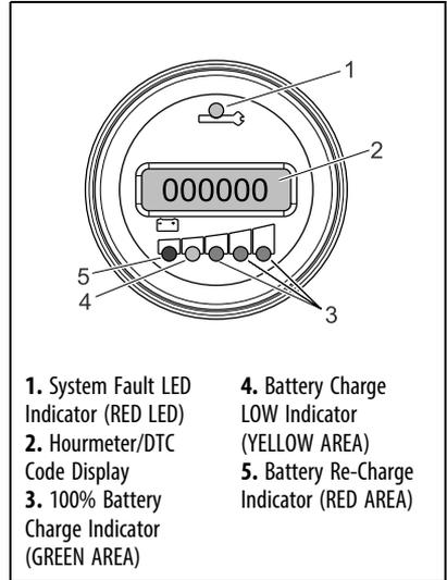
Also located on the MDI are Battery Discharge Indicators (BDI) (3, 4, 5). The three green LEDs indicate the level of charge (voltage) remaining in the batteries.
