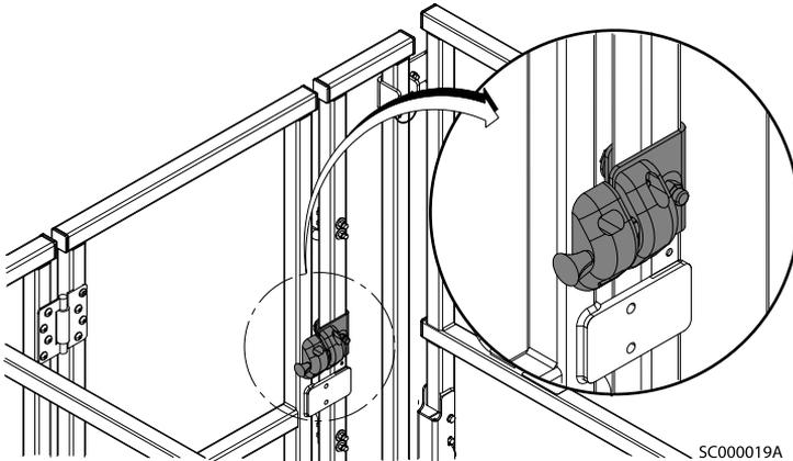
Figure 9. Magnetic Gate Latch Assembly
