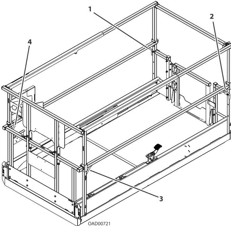
**Figure 3. Lanyard Attach Points**
