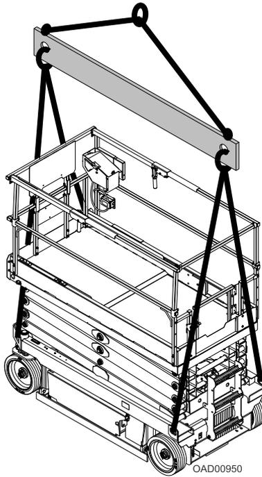
The machine may also be lifted using a spreader bar and four equal length straps or chains capable of supporting the full gross weight of the machine. Lift only using the lifting lugs provided at the four corners of the machine. When transporting the machine, fully lower the platform (stowed position) and secure the machine to the truck or trailer deck. There are two tie-down/lift lugs at the rear of the machine, and two tie-downs and one lifting lug at the front of the machine.
