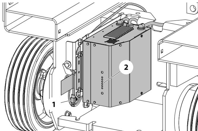
1. AC Voltage Input Cable      2. Charge Indicator LEDs
