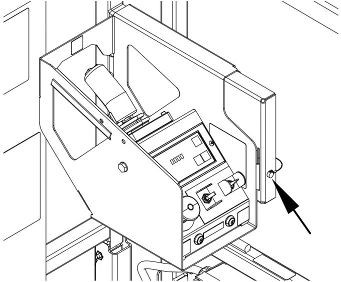
To prevent unauthorized removal, the platform control station can be secured to its mount by replacing the lock pin located on its mounting tab with a keyed or combination lock.
