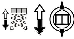
**NOTE:** To ensure proper operation of the desired platform function, move the joystick in the direction of the black or white arrow that matches the color of the arrow on the chassis for the intended direction of travel.
