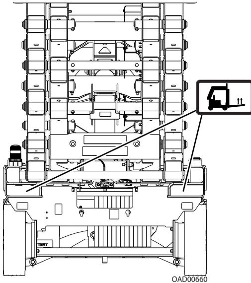
The machine may be lifted using a forklift truck. Lift only using the built-in forklift pockets at the rear of the machine and only with the platform in the stowed position. First adjust the width of the forklift truck lifting tines to fit the machine forklift pockets. Then slide the tines into the forklift pockets and carefully lift machine.
