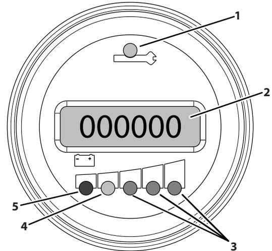
1. System Fault LED Indicator (Red LED)
