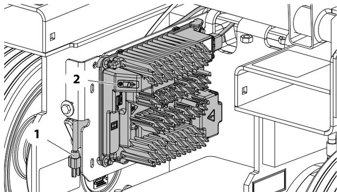
1. AC Voltage Input Plug      2. Charge Indicator LEDs
