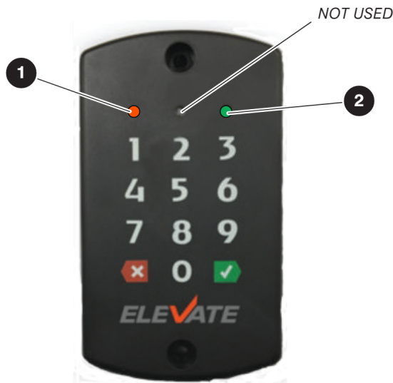
Figure 06 Keypad of the access control unit
