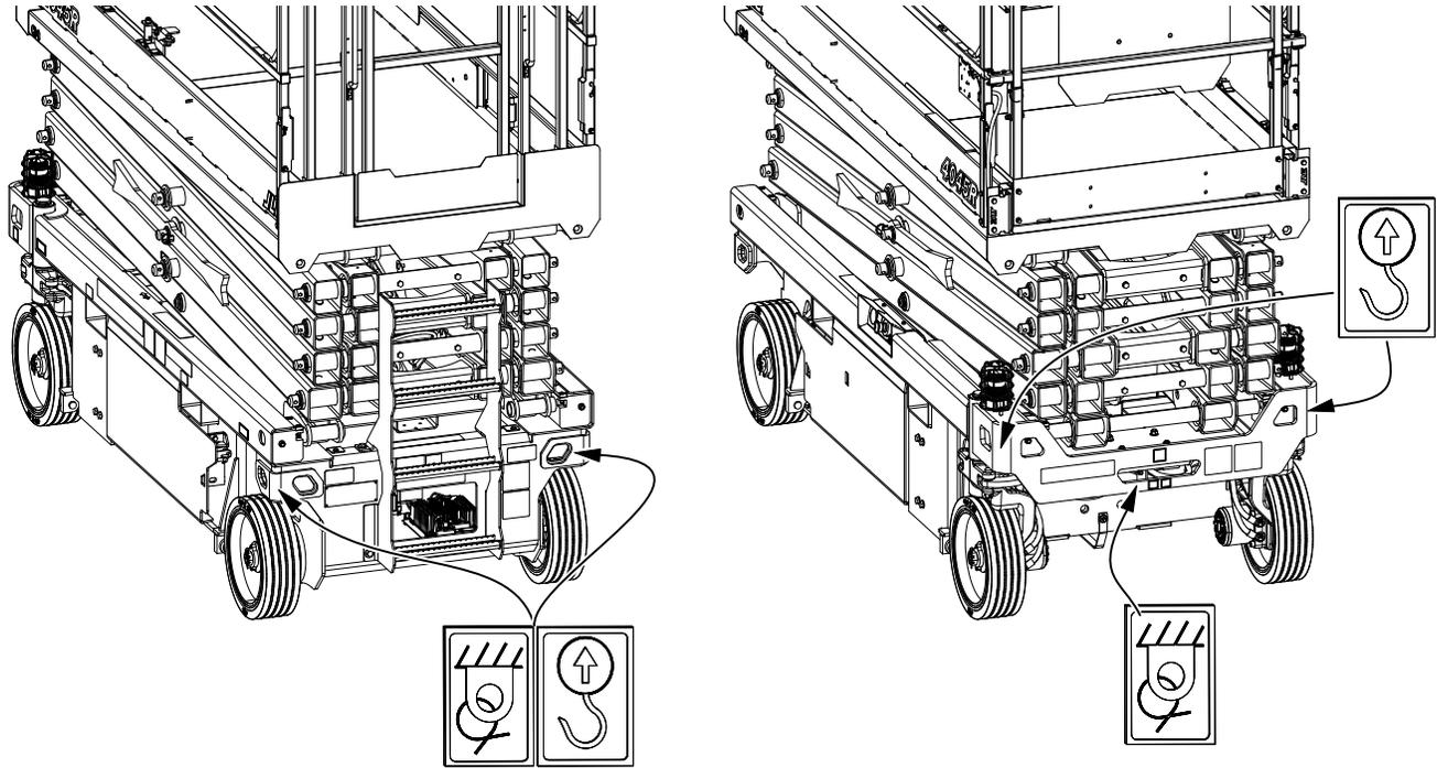
**Figure 3-13. Tie Down and Lift Lug Locations**
