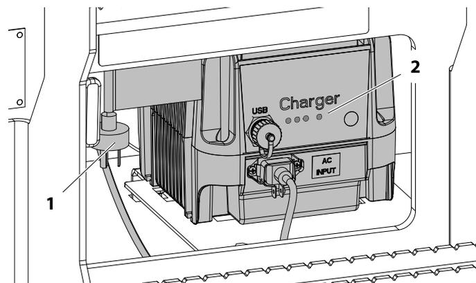
1. AC Voltage Input Cable      2. Charge Indicator LEDs
