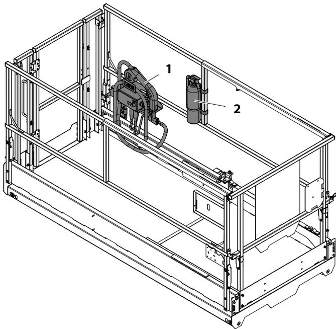
1. QuickWelder Assembly      2. Fire Extinguisher
