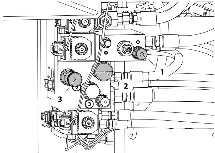
**Figure 3-14. Hydraulic Brakes - Manual Disengage**
