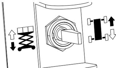
This toggle switch is used to select operation of either the drive or lift function. After selecting a function, the joystick controller must be moved in the proper direction in order to activate that function. Only change the function selected, with the joystick in the neutral position. Otherwise, the function selected will not change until the joystick is returned to the neutral position.
