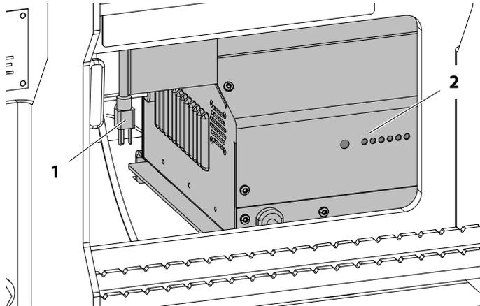
1. AC Voltage Input Cable      2. Charge Indicator LEDs
