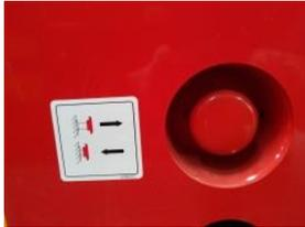
Press the DC power switch, power supply of the whole machine will be disconnected.
