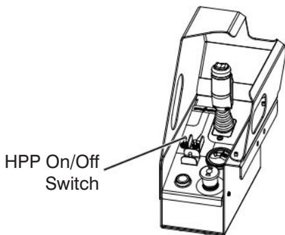
Figure 3-9. Platform Control Console
