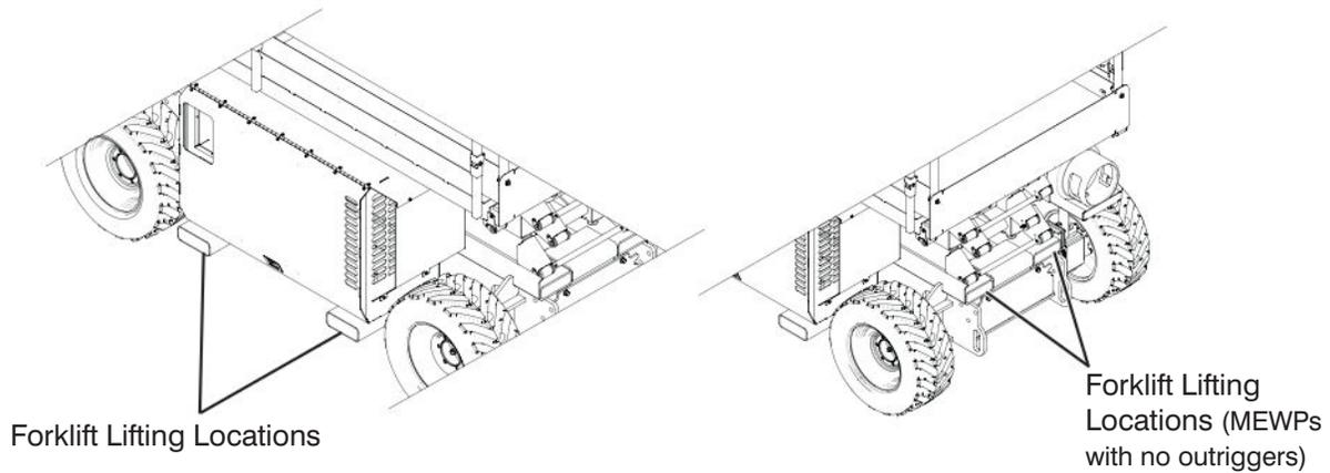
*Figure 3-15. Forklift Lifting Locations*
