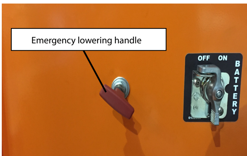
Figure 2-8: Emergency Lowering handle.
