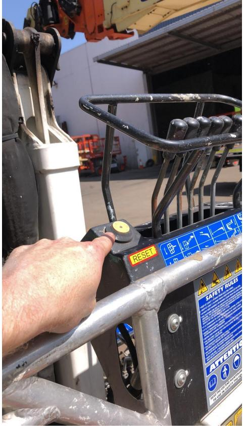
When this button flashes, you have gone out of your safety envelope. Press and hold button, while drawing machine back into its safety parameters. Set machine up closer to the intended job.
