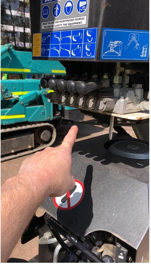
This lever switches between base & basket controls. LEFT=base, RIGHT=basket controls
