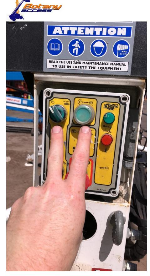
The left switch changes the machine between electric and motor power (left for motor- right for electric) the right switch starts the electric motor. **MACHINE WONT** WORK ON 240v **UNLESS LEAD IS PLUGGED IN AT BASE**, AND **ELECTRIC MOTOR HAS BEEN STARTED**.
