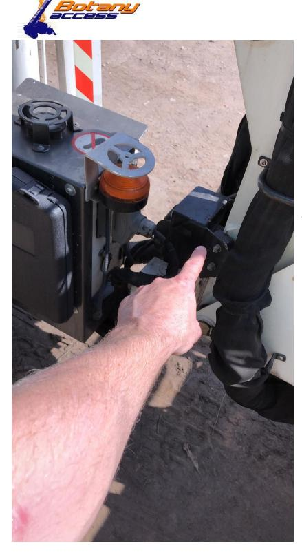
If machine won't drive after stowing machine away, or cuts out while driving, check that the basket jib is hard up against this sensor. This function will still work while the legs are up.
