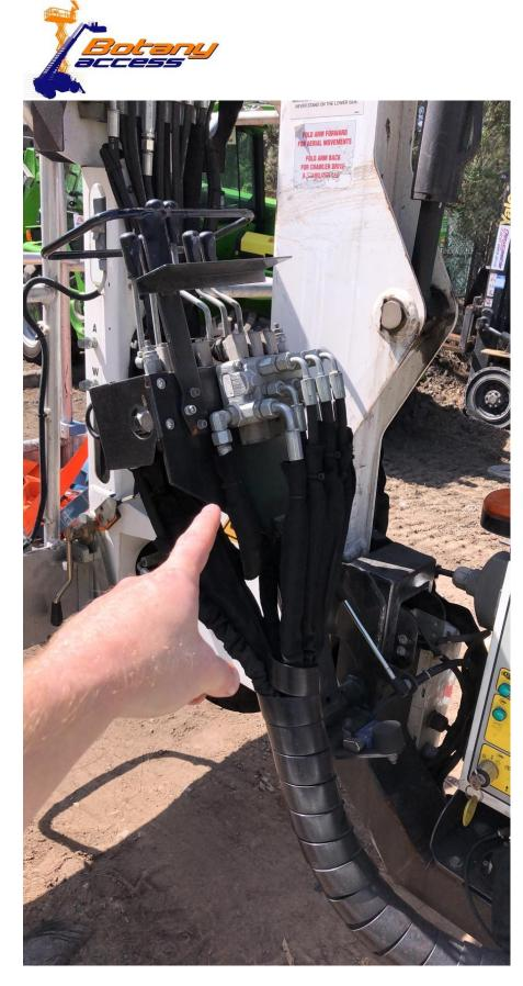
These controls need to be brought forward before you can operate the machine from the basket.
